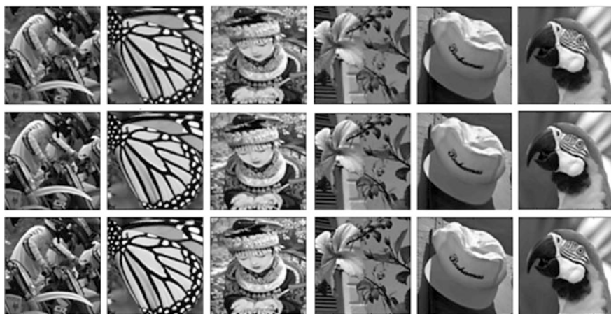
Fig. 5.15 Processed images with the decoupled gradient algorithm. The scale factors are: 4\times for the top row of images, 3\times for the second row of images, and 2\times for the row of images at the bottom
