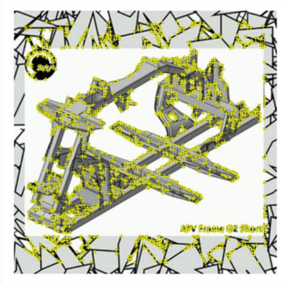
Fig. 3.11 Fingerprints obtained by Vuforia for short marker
