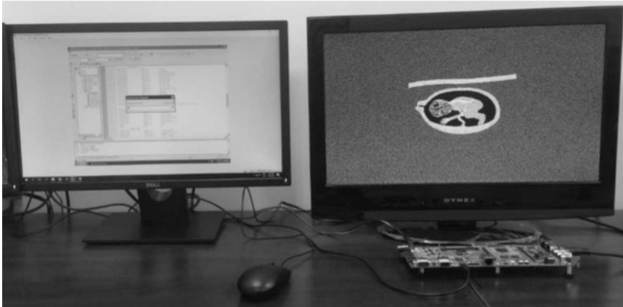
Fig. 1.4 System configuration: code composer software, interface to the DM6437 EVM and the display unit
