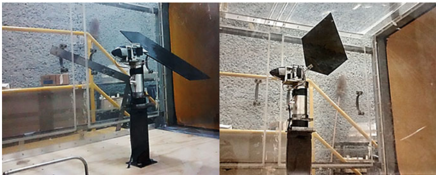
Fig. 14.8 Test two and three. Figure shows the attitude of the stabilizer due to the bank (left) and tilt (right) motions
