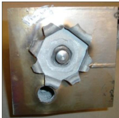
Figure 5.7 Laminated armor after ballistic testing. The part was built using ultrasonic additive manufacturing (UAM). Source: Courtesy of Mark Norfolk, Fabrisonic LLC.
