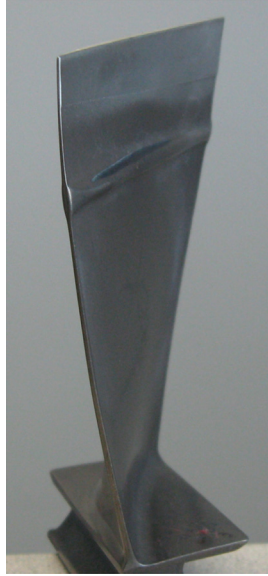
Figure 6.3 Vane tip repair using the DMD process. 4 Source: Courtesy of DM3D Technology.
