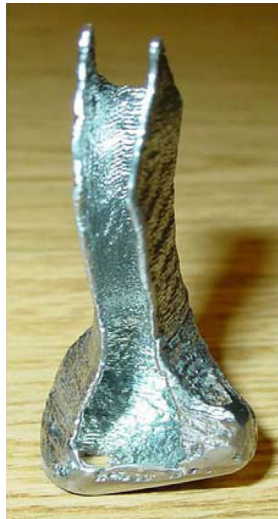
Figure 6.5 Ti-6Al-4V scaffold which was produced by the DMD process. 7
