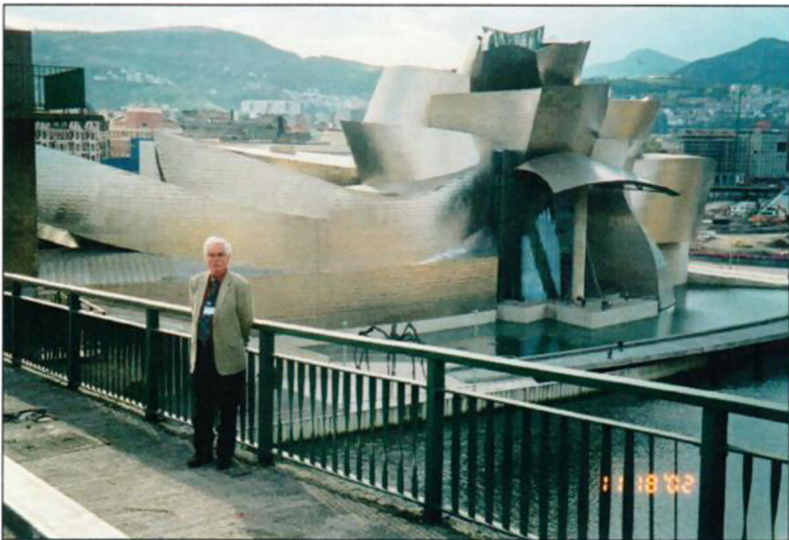
Figure 1.3 Author Dr. F.H (Sam) Froes is shown in front of The Guggenheim Museum in Bilbao, Northern Spain, which is sheathed with titanium sheet.
