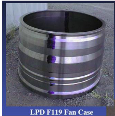
Figure 5.4 Fan case produced by adding features with AM (laser aided directed energy deposition) to a forged perform. Source: Courtesy of Jim Sears.
