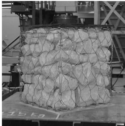
Figure 1. Geocomposite cell filled with natural stones used for civil engineering structures.
