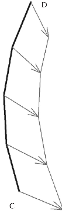
Figure 11. Top bench support displacement at the end of construction (max: 17 cm).
