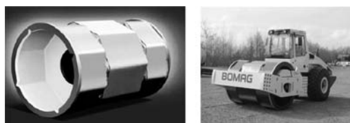
Figure 11. Polygonal drum and in a single drum roller BOMAG BW 226 DI with polygonal drum.
