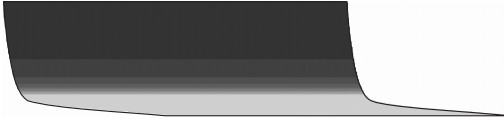
Figure 5. Contour plot of the void ratio within a reinforced granular layer after a horizontal reinforcement displacement of u_{1R}/h_0 = 1.4 ( d_{50} = 1 mm).
