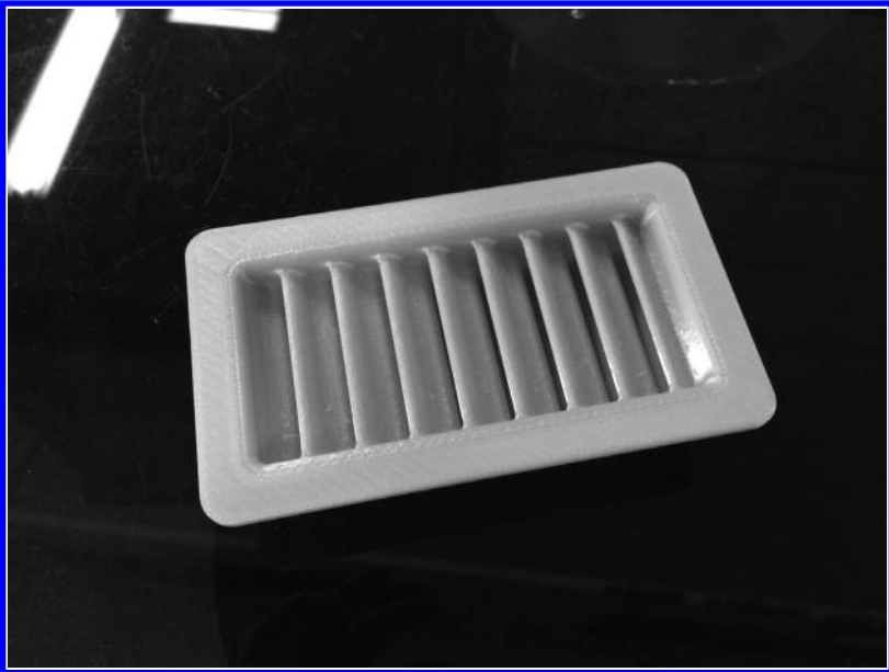
FIGURE 9.2 Air guiding grate made from Ultem 9085 using Stratasys FDM™. (Copyright Rapid Prototype and Manufacturing, LLC, Avon Lake, Ohio, 2014.)
