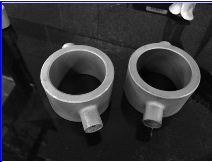
FIGURE 9.16 Pair of water cooling channels made from MS1 on an EOS DMLS™ platform. (Copyright Rapid Prototype and Manufacturing, LLC, Avon Lake, Ohio, 2014.)
