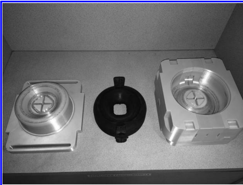
FIGURE 9.9 (See color insert.) Injection mold core and cavity set for thermoplastic elastomer molding made from Ultem 9085 using Stratasys FDM™. (Copyright Rapid Prototype and Manufacturing, LLC, Avon Lake, Ohio, 2014.)
