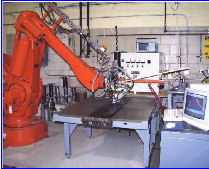
FIGURE 2.25 A typical ATP setup used. (Data from Yarlagadda, S., Automated Tow Placement of Composites, 2014.)
