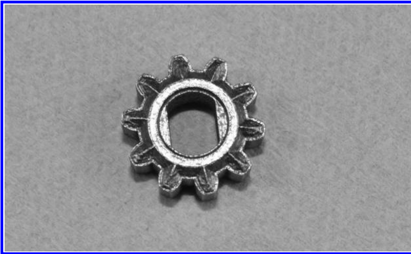
FIGURE 9.15 Functional gear prototype made from PH1 stainless steel on an EOS DMLS™ platform. (Copyright Rapid Prototype and Manufacturing, LLC, Avon Lake, Ohio, 2014.)
