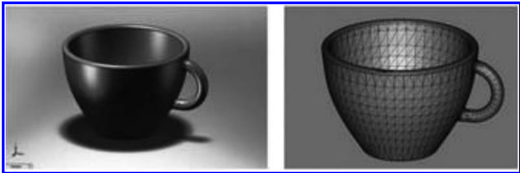
FIGURE 4.6 On the left side a conventional CAD file. On the right side a STL file with triangles. (Data from Gibson, I. et al., Additive Manufacturing Technologies, Rapid Prototyping to Direct Digital Manufacturing , Springer-Verlag, 2010.)
