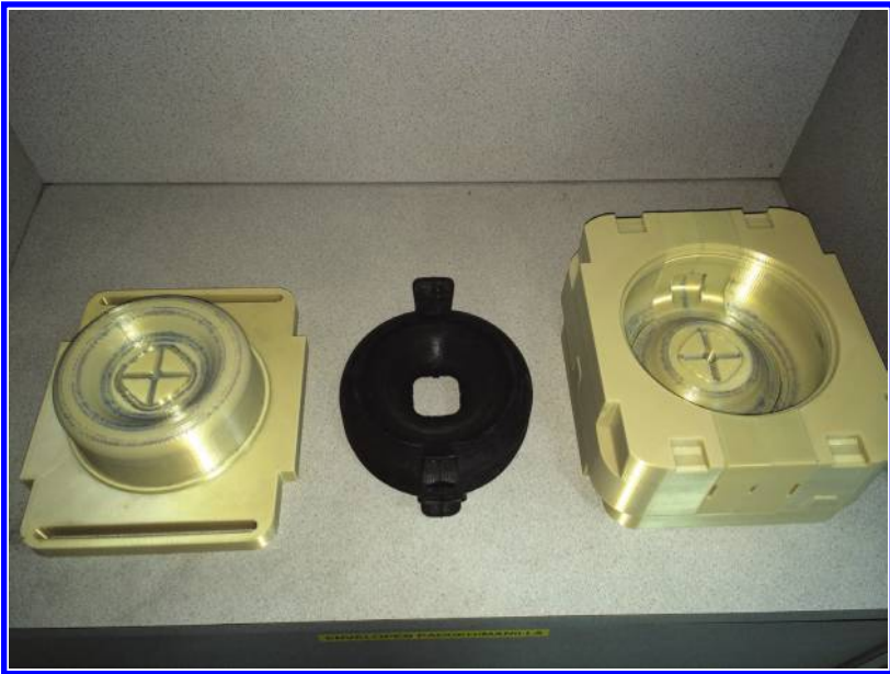
FIGURE 9.9 Injection mold core and cavity set for thermoplastic elastomer molding made from Ultem 9085 using Stratasys FDM™. (Copyright Rapid Prototype and Manufacturing, LLC, Avon Lake, Ohio, 2014.)
