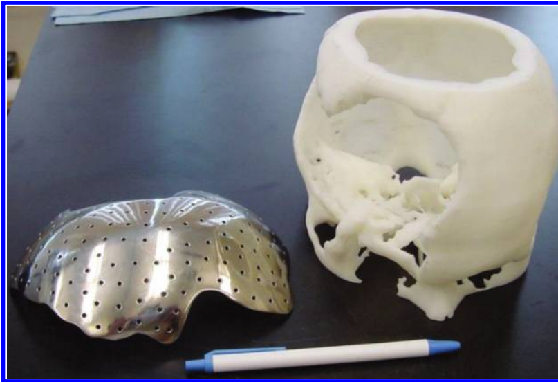
FIGURE 14.2 LENS processed craniofacial Ti implant and FDM processed polymer prototype of the skull with large defect.
