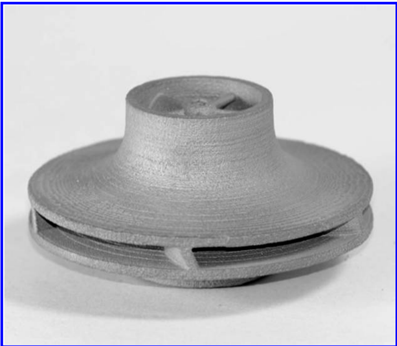
FIGURE 9.19 Example of a hydraulic fluid moving impeller for a heavy truck application made from 410 stainless steel–bronze composite using binder jetting on an ExOne M-Flex platform. (Copyright Rapid Prototype and Manufacturing, LLC, Avon Lake, Ohio, 2014.)
