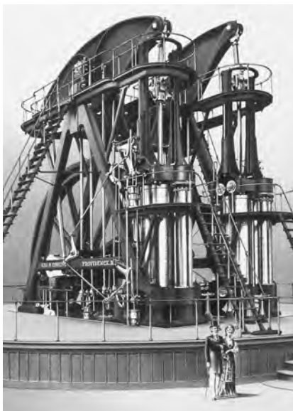
The Corliss steam engine of 1876. Engineers discovered that no matter how they designed their heat engines, not all of the heat produced could be converted into work. (Science Museum, London/Topham-HIP/The Image Works)
