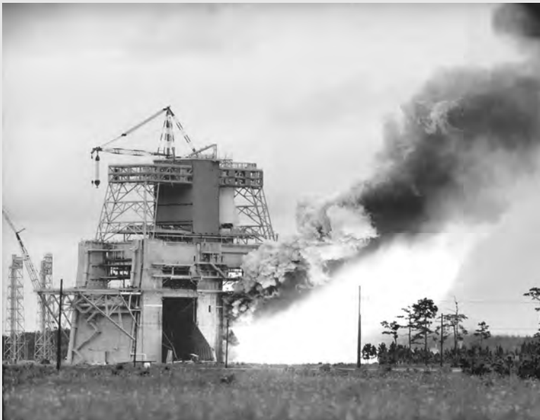
Test firing of the Saturn rocket engine, an especially dramatic form of combustion (Courtesy of National Aeronautics and Space Administration)
