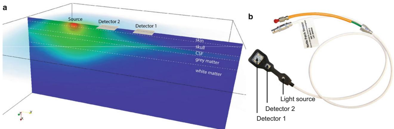
**Fig. 2** Monte Carlo simulation of light propagation at 800 nm in a layered head model (a). The light intensity is shown in a logarithmic scale. Light guiding occurs in the cerebrospinal fluid layer, which has a slightly higher refractive index than the surrounding tissue. On
