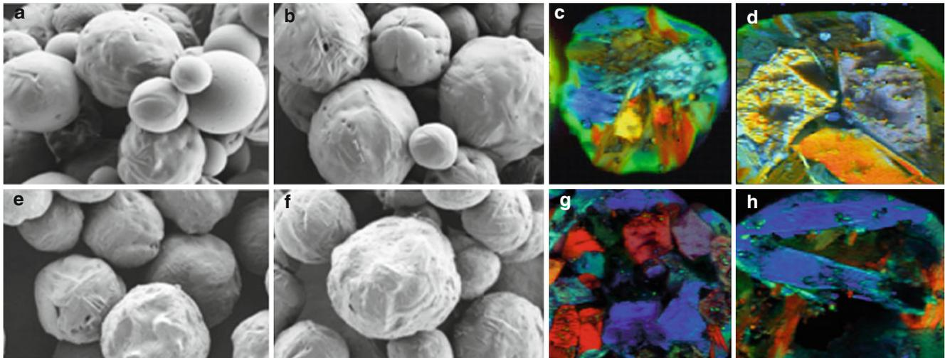
**Fig. 1** Scanning electron microscopy and Raman spectroscopy of an example of one formulation of nimodipine microparticles. Scanning electron microscopy (a, b) and Raman spectroscopy (c, d, red is form 1 of nimodipine, green is amorphous nimodipine, and blue is form 2 of nimodipine) at baseline. After attempted forced degradation at 30–35 °C
