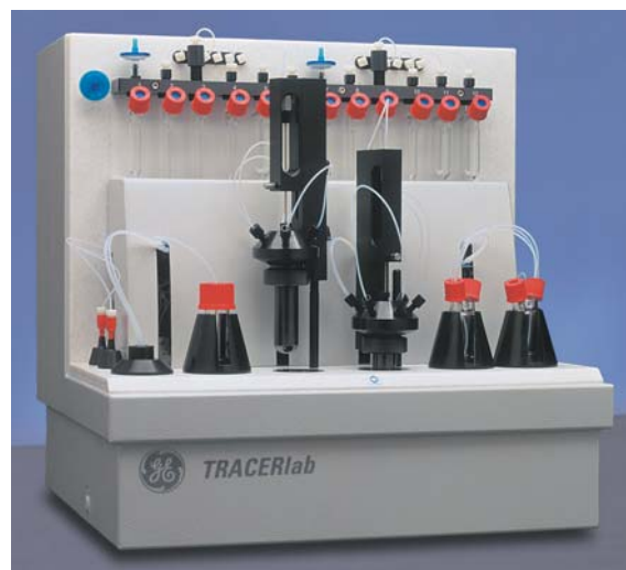
Figure 32.25 Automated 2-[ ^{18}\text{F} ]fluoro-2-deoxy-D-glucose ( ^{18}\text{F} -FDG) synthesis unit
