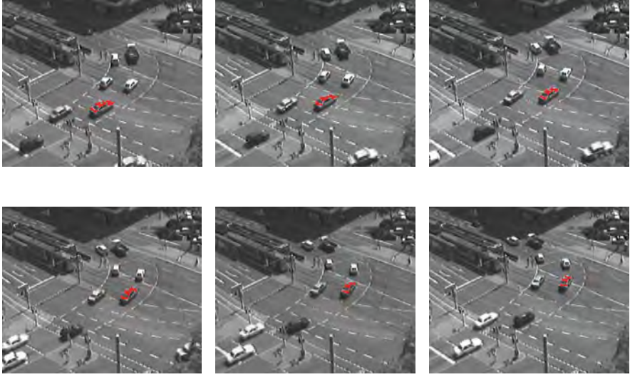
Fig. 1.3 Extract of 50 images with slow changes. One car is marked in the first image and then the discrete algorithm detects it in the subsequent images while passing the crossroads
