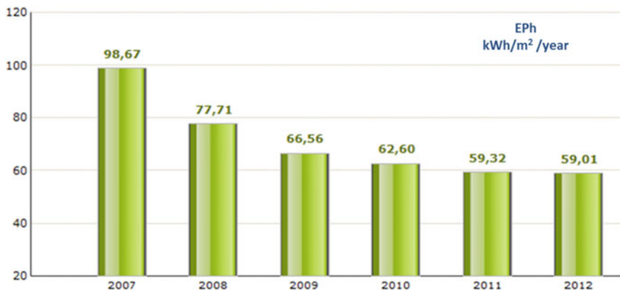
Fig. 18.3 Trend of energy demand per unit of space for new buildings in Lombardy
