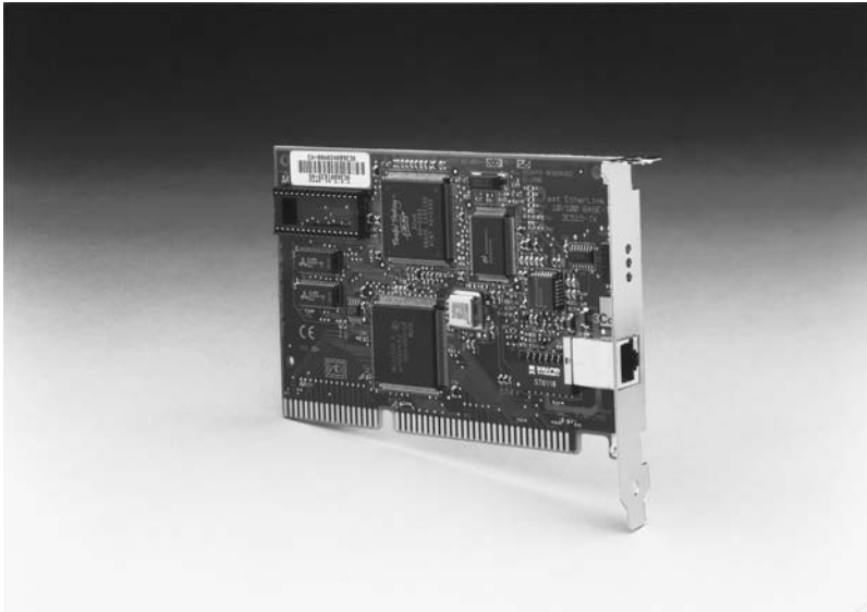
Figure 3.42 The 3Com Corporation Fast Etherlink TX NIC supports the use of the ISA bus. (Photograph courtesy of 3Com Corporation.)
