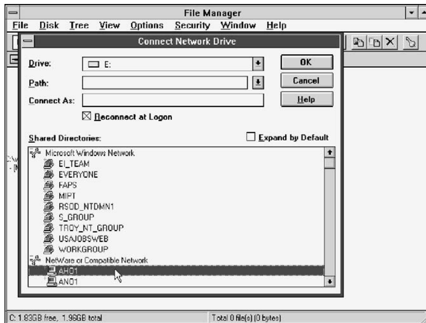
Figure 5.24 Viewing devices on both a Windows and a Novell network through the Windows NT File Manager.
