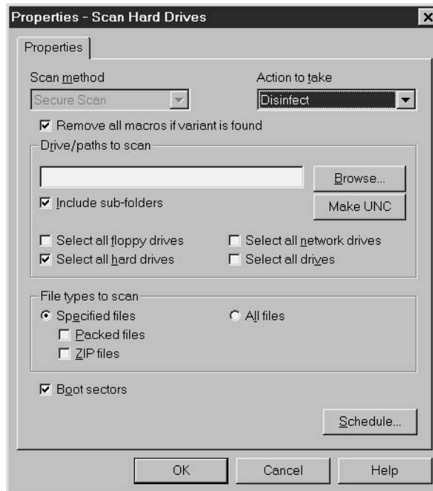
Figure 9.27 The Command AntiVirus Properties dialog box provides users with the ability to control both when and how a virus scan is performed as well as the actions to occur if infected files are discovered.
