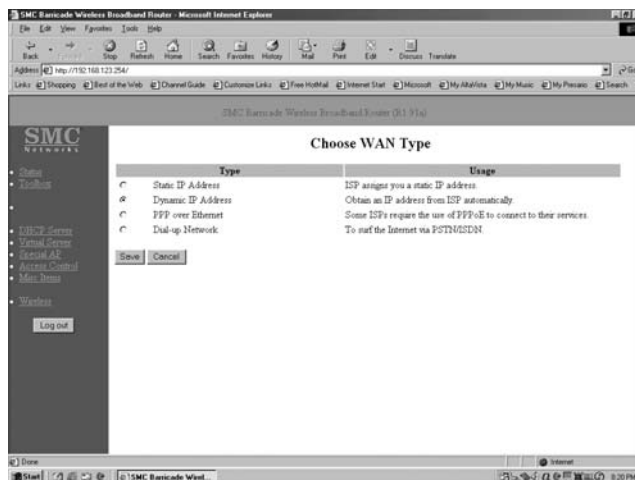
Figure 8.20 The primary setup entry permits a user to define how the SMC Networks Barricade broadband router will be connected to the Internet.
