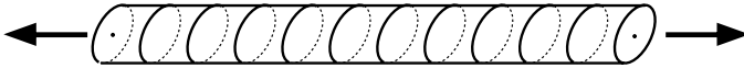
Fig. 2.5. Configuration of a doubly hinged, initially cylindrical rod undergoing a shear instability. The corresponding instability for a doubly welded rod is illustrated in Fig. 2.6.
