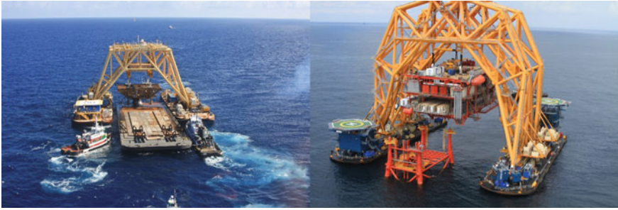
Fig. 2.53 Bottom Feeder with lifting capacity of 4000 tons ( left ) and VB 10,000 with lifting capacity of 7500 tons ( right ) (courtesy of Versaba, Inc.)
