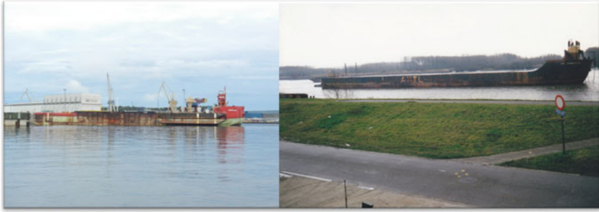
Fig. 6.12 The two barges being used in the Hibernia catamaran floatover. On the left is Neptune's Goliat 10 and on the right is AMT Transporter. The two are not sister vessels with the same size and design (courtesy of HMDC)
