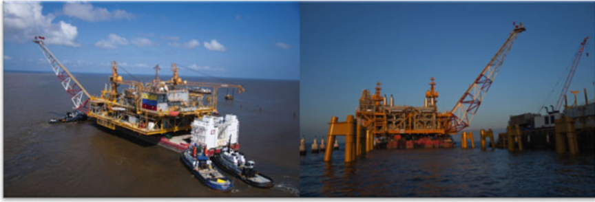
Fig. 2.55 Corocoro CPT (Central Production Facility) project was in the 5 m water depth field (courtesy of ConocoPhillips)
