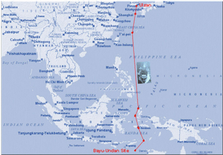
Fig. 10.7 The topsides of CQU and DPP topsides of the Bayu Undan projects were built in Ulsan South Korea and were transported the offshore site located at Timor Sea, Australia. The voyage was more than 2900 nautical miles (Based on Bayu Undan Project information)
