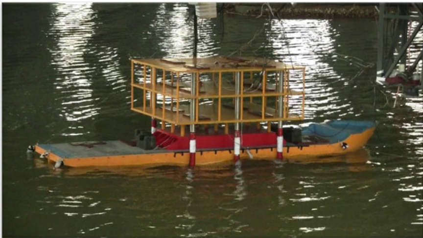
Fig. 8.18 Model test of pre-mating condition for Chengdao Central Platform III of Sinopec (credit to the project)
