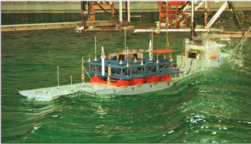
Fig. 8.17 Model test of transportation condition for Bayu Undan project (credit to Bayu Undan project)
