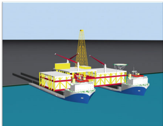
Fig. 6.17 Demonstration of loading out the topsides longitudinally on the parallel moored two vessels to form a catamaran for floatover operation
