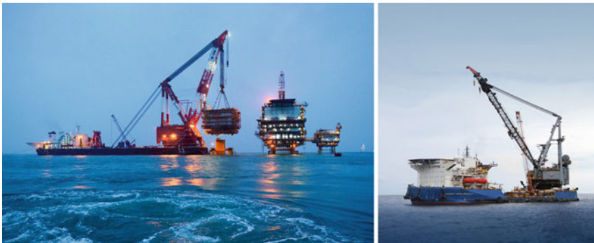
Fig. 2.49 HLCVs. On the left is Blue Whale of COOEC hoisting the largest offshore oil wellhead platform module in Bohai Sea China. On the right is the McDermott DB-50 equipped with DP system (courtesy of CNOOC and McDermott)
