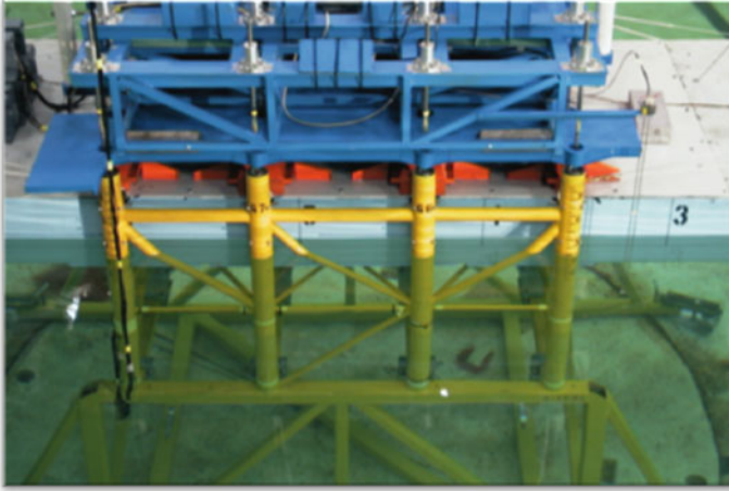
Fig. 8.19 Model test of mating condition for Bayu Undan project (credit to Bayu Undan project)
