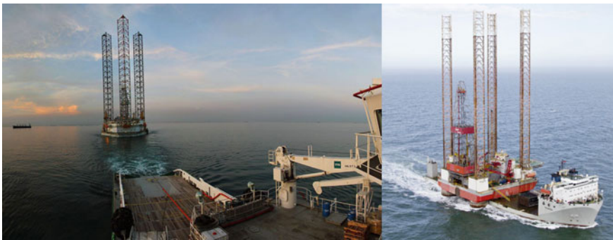
Fig. 2.5 Transportation of jack-up platforms: the left shows “wet tow” by a tug boat and the right one shows “dry-tow” by a semi-submersible HLV (courtesy of COSL. and COSCO)
