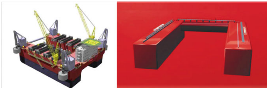
Fig. 2.59 Example of vessel concepts for catamaran. On the left is a conceptual design of OCDV (Offshore Construction and Decommissioning Vessel) by Master Marine AS. On the right is the catamaran vessel concept from student team of the University of California, Berkeley in 2002 (courtesy of Master Marine AS and UC Berkeley, Ocean Engineering) [31, 32]
