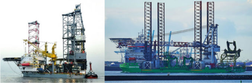
Fig. 2.2 On the left is the three leg Jack-up drilling rig JU2000E of COOEC and on the right is the Jack-up offshore supporting vessel Innovation with four legs (courtesy of Shanghai Waigaoqiao Shipbuilding and Wikimedia commons respectively)
