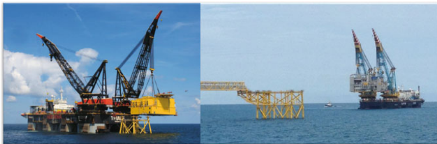
Fig. 1.12 Large SSCV's. On the right is HMC's Thialf of which the nominal lifting capacity is 14,200 t and on the left is SAIPEM 7000 with nominal lifting capacity of 14,000 t (Courtesy of HMC and Saipem)
