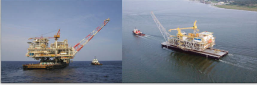
Fig. 1.20 The topsides were transported to the mating sites: on the left the barge was towed to the offshore site and on the right the topsides was towed to KOS yard (Credit to the BP Lan Tay and the Chevron Blind Faith projects)
