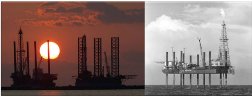
Fig. 2.4 On the left , it showed two different designs of jack-up drilling rigs waiting in Fourchon channel—one with triangular hull and lattice legs and the other with four columnar legs and a rectangular hull; The right photo is the British jack-up drilling rig with ten legs ( Sea Gem ) (courtesy of Houston Chronical and Duke Wood Oil Museum respectively)
