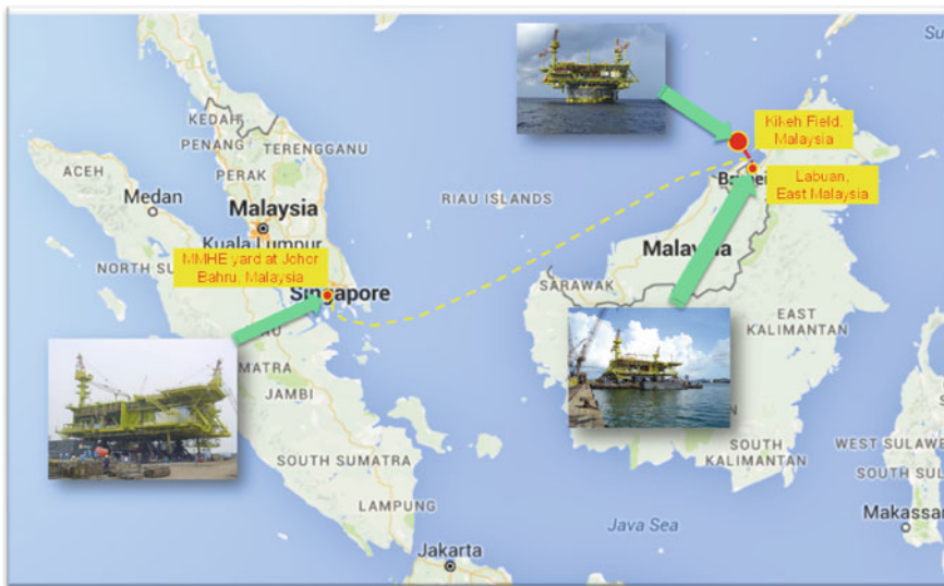
Fig. 6.16 Illustration of the process of catamaran floatover preparation of Kikeh spar. The topsides was transported by a single barge UH336 from the fabrication yard at MMHE’s yard at Johor Bahru, Malaysia to the installation operation base at Labuan, East Malaysia, as indicated by the yellow dash line. The topsides and the two floatover-barges then formed a catamaran which is towed to the mating site of Kikeh spar (courtesy of Murphy Oil Corporation and Technip)
