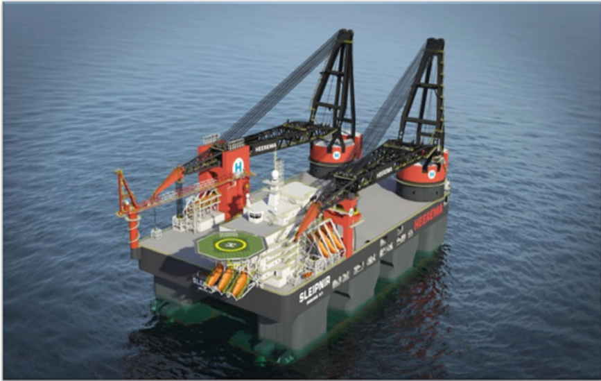
Fig. 3.2 HMC have been planning to build a new SSCV with even higher capacity than SSCV Thialf. The new vessel Sleipnir will be equipped with twin heavy lifting cranes, each of them with lifting capacity of 10,000 Mt at a radius of 48 m (courtesy of HMC)
