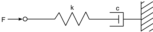
FIGURE 10.3 Schematic representation of a series combination of a spring and a damper.
