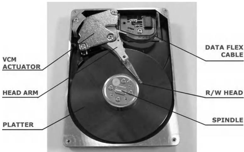
Figure 9.1. An HDD with a VCM actuator
