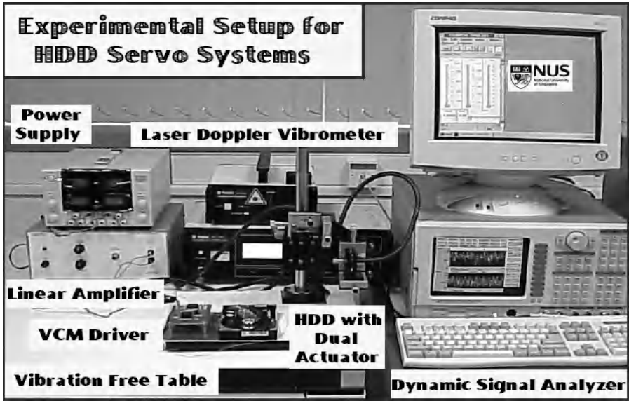
Figure 1.7. Implementation setup for HDD servo systems
