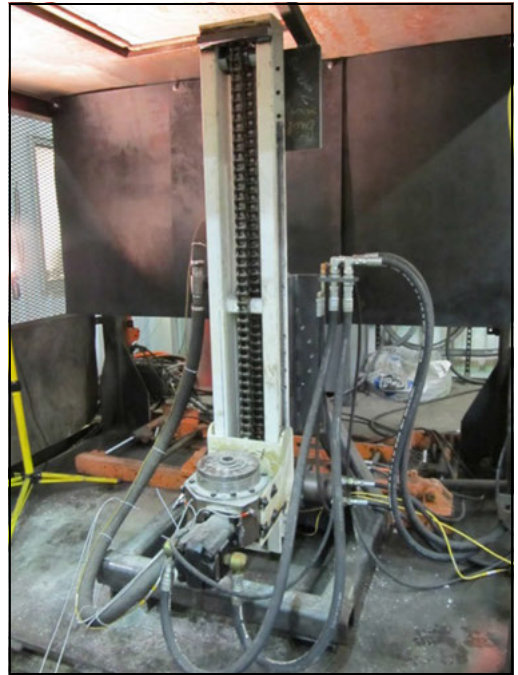
Figure 1. J.H. Fletcher & Co. instrumented roof bolter setup
