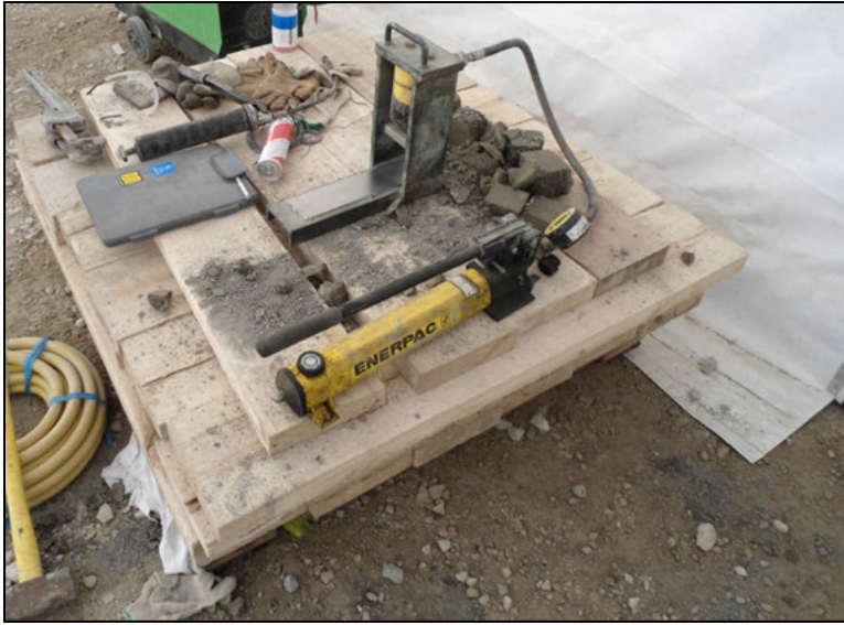
Figure 2. End beam testing apparatus
