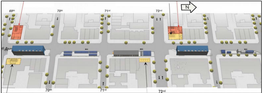
Figure 10. Aerial view along 2nd Avenue after Muck Houses had been installed in mid-2011 at 69th and 72nd Streets. The integrated mucking systems were critical to the schedule and, therefore, overall success of the project.
