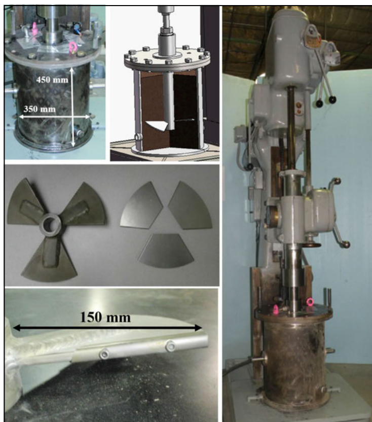
Figure 1. Penn State soil abrasion testing device: cylindrical chamber, device overview; propeller and metal covers
