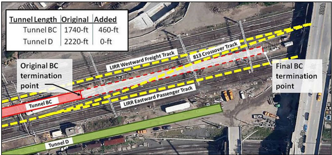
Figure 1. B/C and D Base Contract tunnel lengths and in place railroad infrastructure
