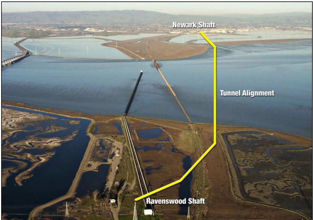
Figure 2. Aerial view of the Bay Tunnel alignment
