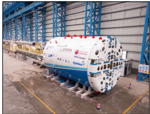
Figure 5. First of two San Francisco Central Subway EPBs with mixed ground tool configuration
