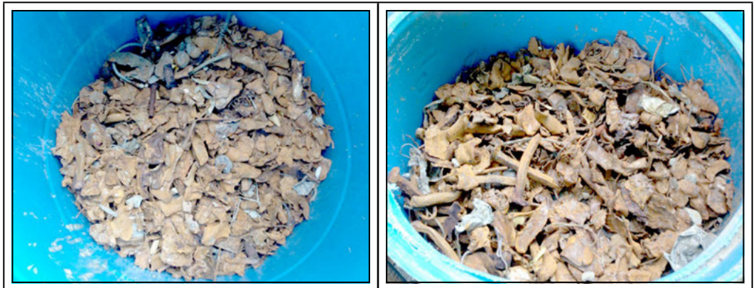
Figure 6. Metals extracted by MTBM collected at separation plant
