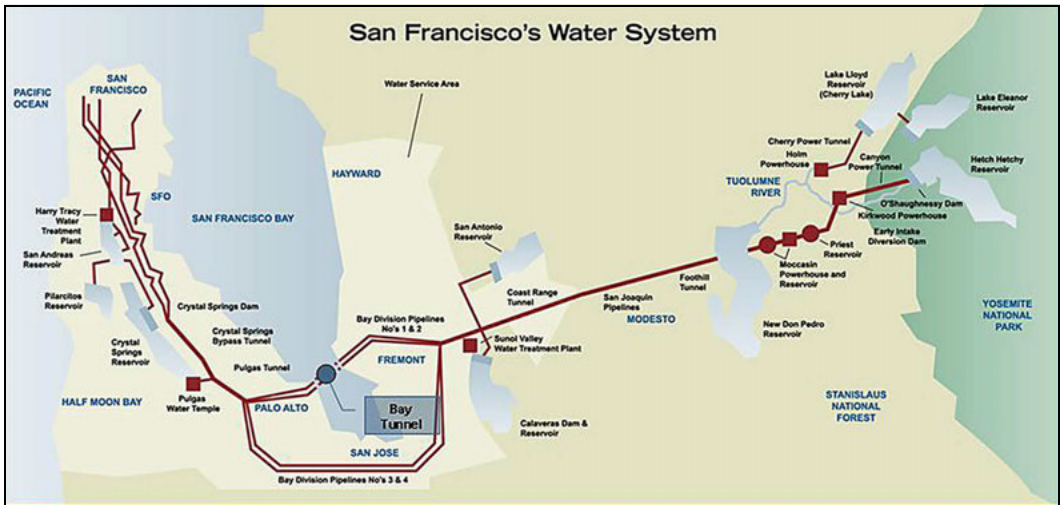
Figure 1. Schematic diagram of the SFPUC's water distribution system
