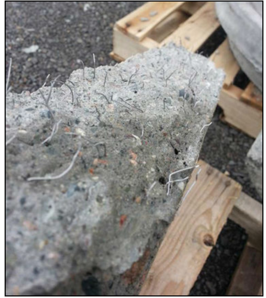
Figure 7. Steel fiber content of a broken RDP after being tested
