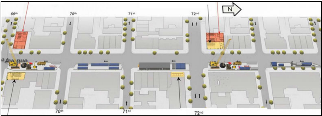
Figure 9. Aerial view along 2nd Avenue as the shaft sinking work got underway in late 2010 at 69th and 72nd Streets. Large cranes were used to service the shafts with marginal productivity due to the physical confinements of the site.
