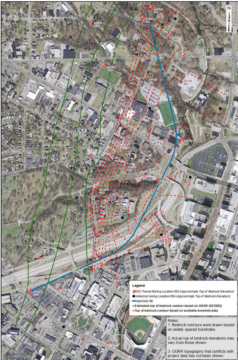
Figure 6. Selected OC1 storage and conveyance tunnel P.E.R. alignment with estimated bedrock contours from P.E.R. investigations
