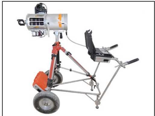
Figure 1. Example of stop & go (static) scanning system
