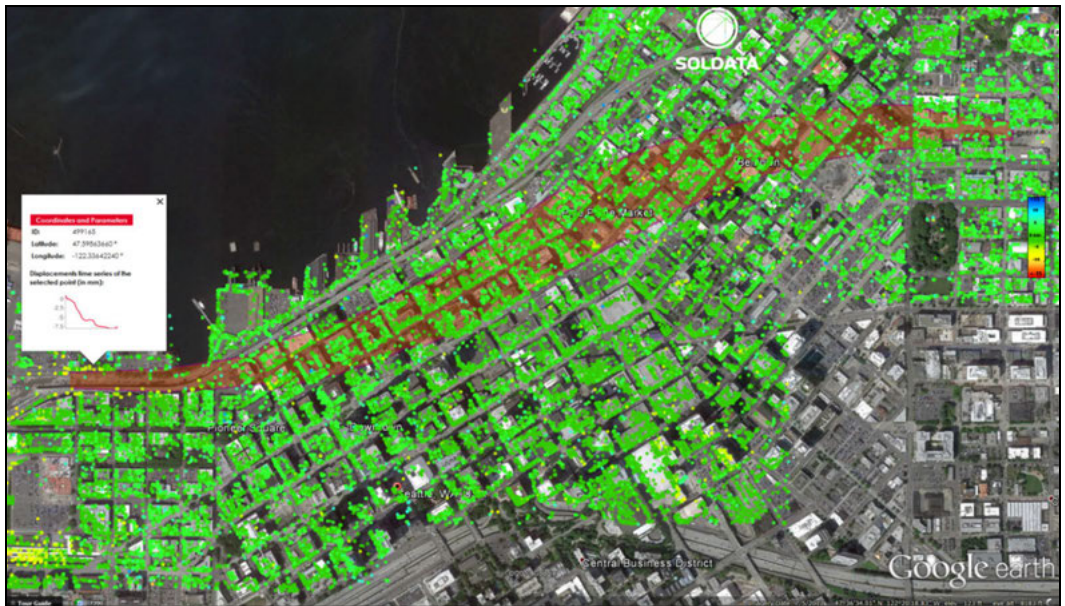
Figure 1. Overview of radar interferometry satellite coverage overlapping the ZOI
