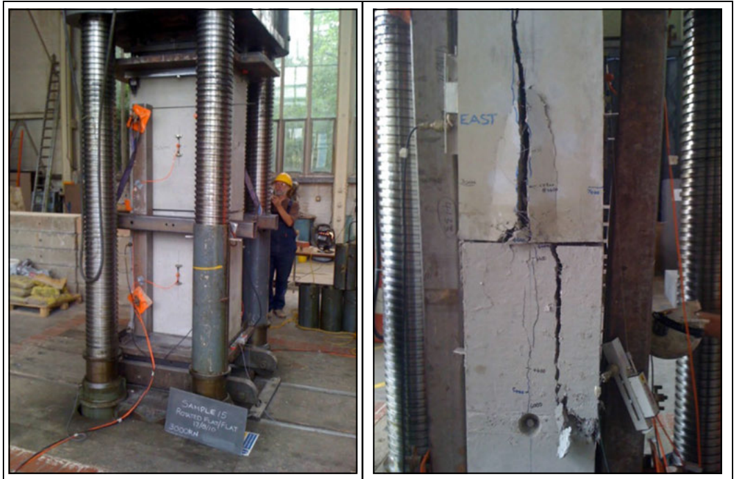
Figure 8. Full-scale load testing of tunnel segmental primary linings
