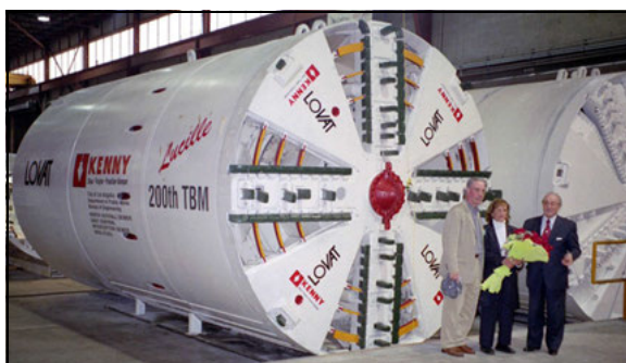
Photo 6. Earth pressure balance TBM (Courtesy of J. Critchfield)
