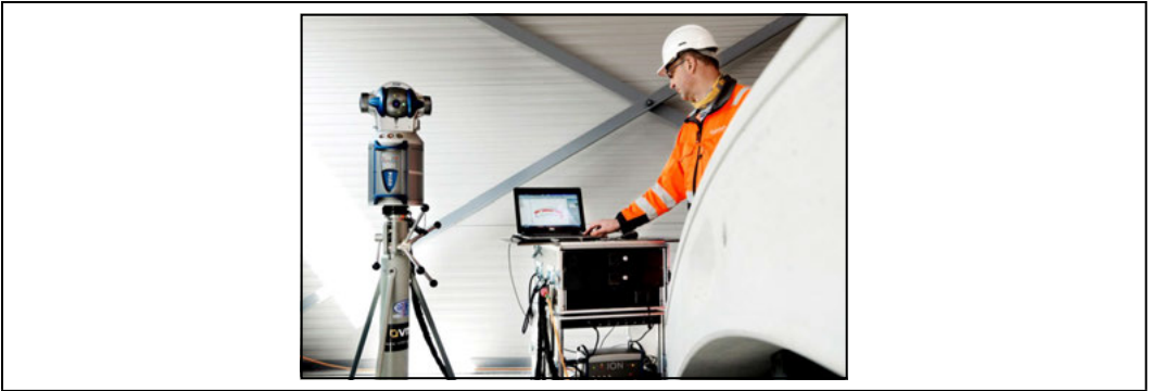
Figure 5. 3D full plane measurement using LaserTracker instrument
