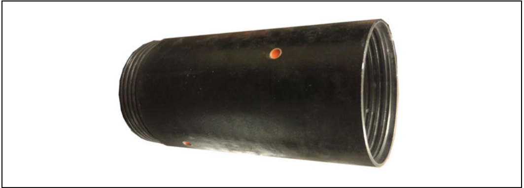
Figure 9. Sample length of 6-inch diameter steel SPP
