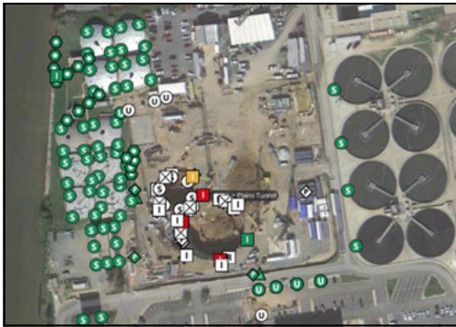
Figure 6. Instruments at BPAWWTP site
