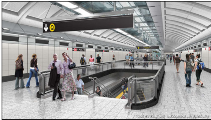
Figure 3. Architectural rendering of station mezzanine with exposed coffers in cavern final lining
