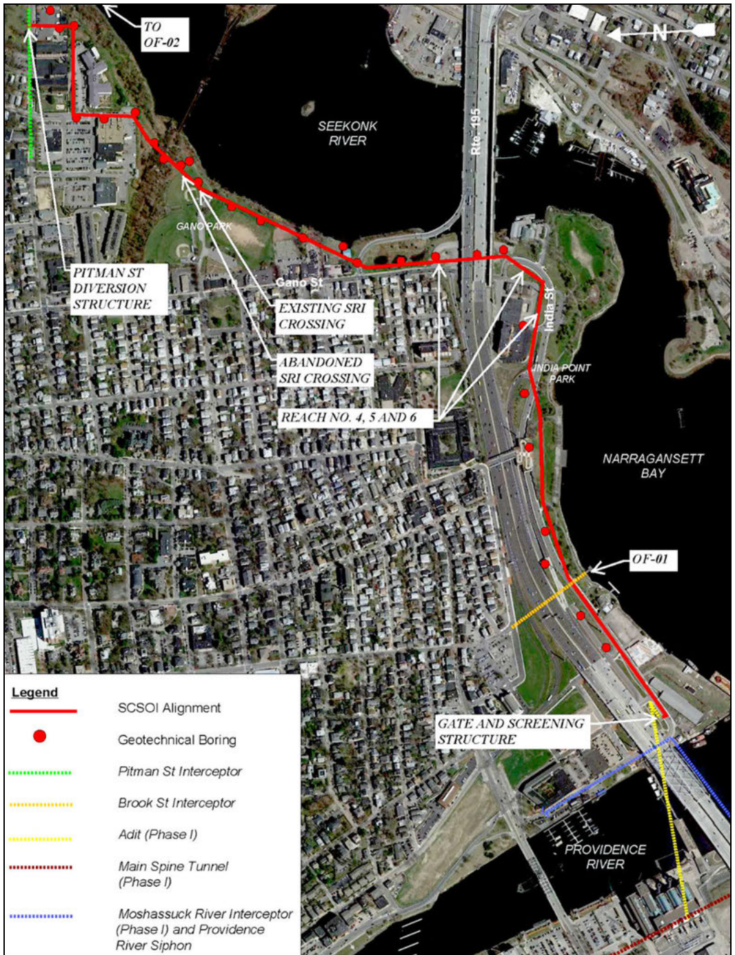
Figure 1. Pipeline alignment and boring locations
