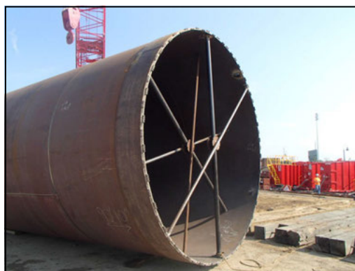
Figure 21. Overburden casing with carbide steel cutting teeth
