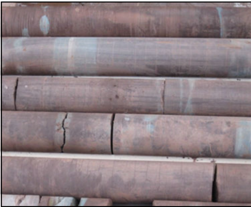
Figure 11. Intact rock cores with breaks from sampling equipment
