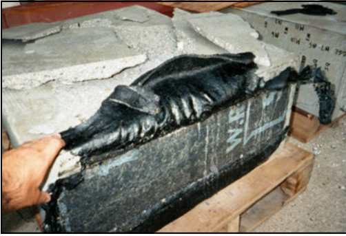
Figure 8. Mastic packer material test (Arrowhead project)
