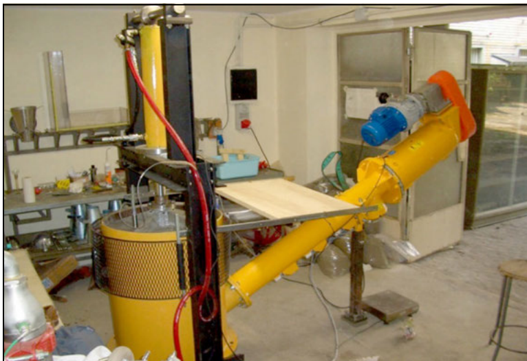
Figure 2. Testing fixture. Treated sample is placed in barrel on left and subjected to pressure and extracted from barrel through screw conveyor on right (Photo courtesy of Mapei-UTT).
