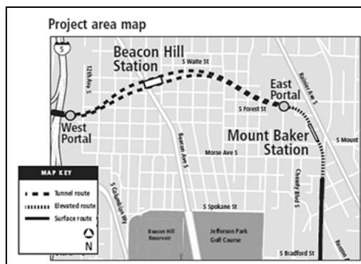
Figure 2. Construction of the station began in March 2005 and was completed in July 2009. Obayashi Corporation was the general contractor and twin tunnels were excavated by a TBM named the “Emerald Mole.”
