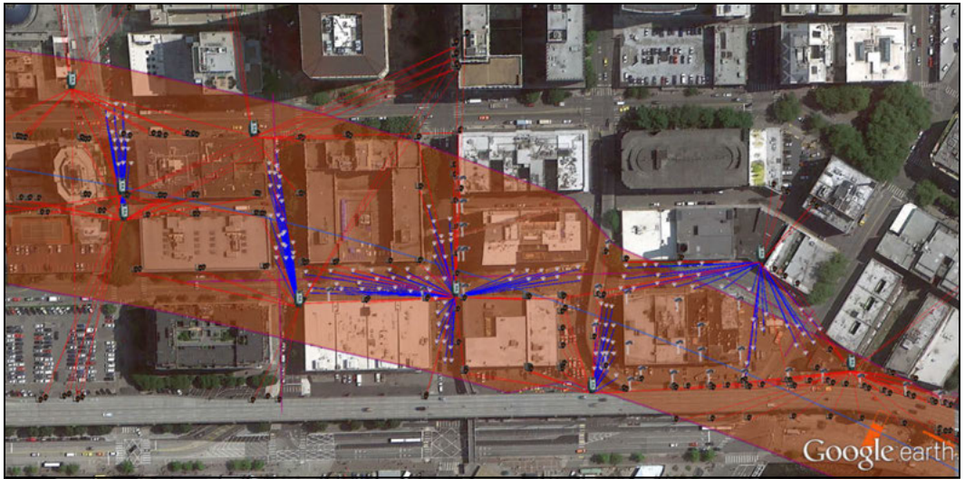
Figure 1. Layout of AMTS and prisms on the south end of the alignment for the SR-99 Tunnel Project
