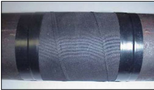
Figure 7. 2-inch diameter steel SPP with protection over the grout port
