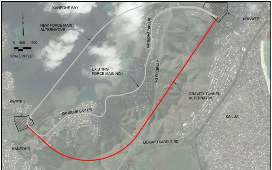
Figure 1. Force main replacement alignment alternatives
