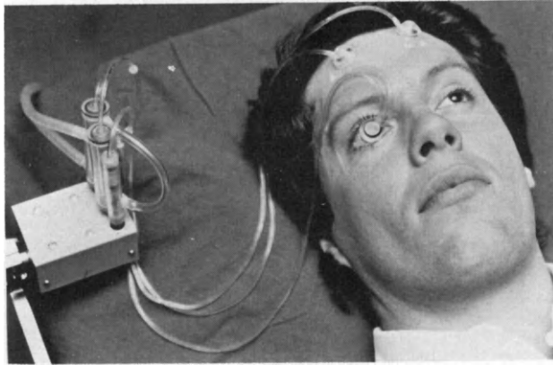
Fig 4. Arrangement for direct SP registration.
