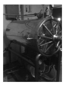
steam from circulating freely around the contents and impedes the full contact that is necessary. The holding time varies from 10 minutes for light loads to 40 minutes for heavy or bulky ones; the average time being 20 minutes.
