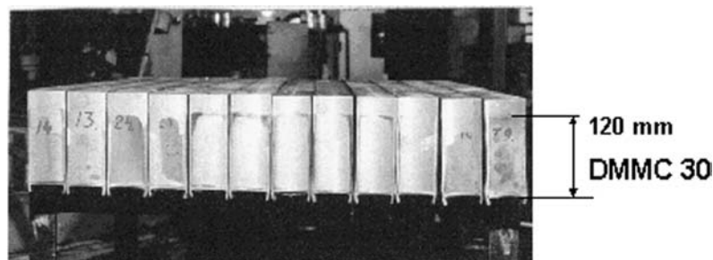
Figure 20 The weldable construction steel clad with MMC in the HIPed high temperature erosion shield blocks (courtesy of Metso Powdermet Oy).
