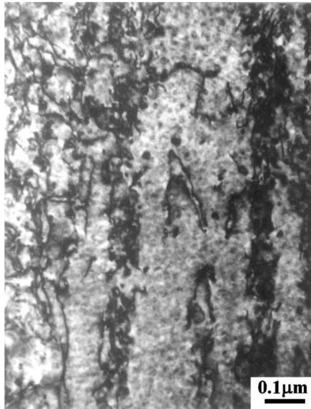
Figure 5 Occurrence of planar slip in Al-Li alloys due to the shearing of \delta' precipitates.
