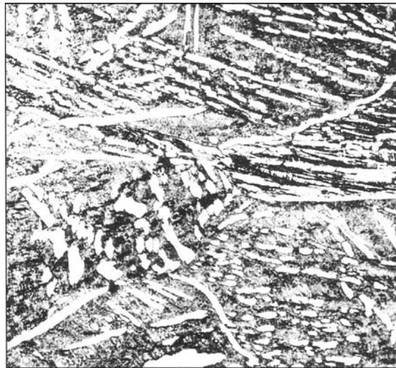
Figure 29 Blocky alpha with grain boundary alpha decorating prior beta grain boundaries. Note: strain porosity associated with both types of alpha. Background is transformed beta.
