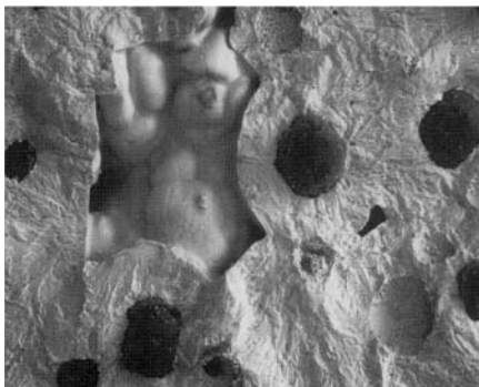
Figure 24 Microshrinkage in ductile iron. (From Ref. 2.)
