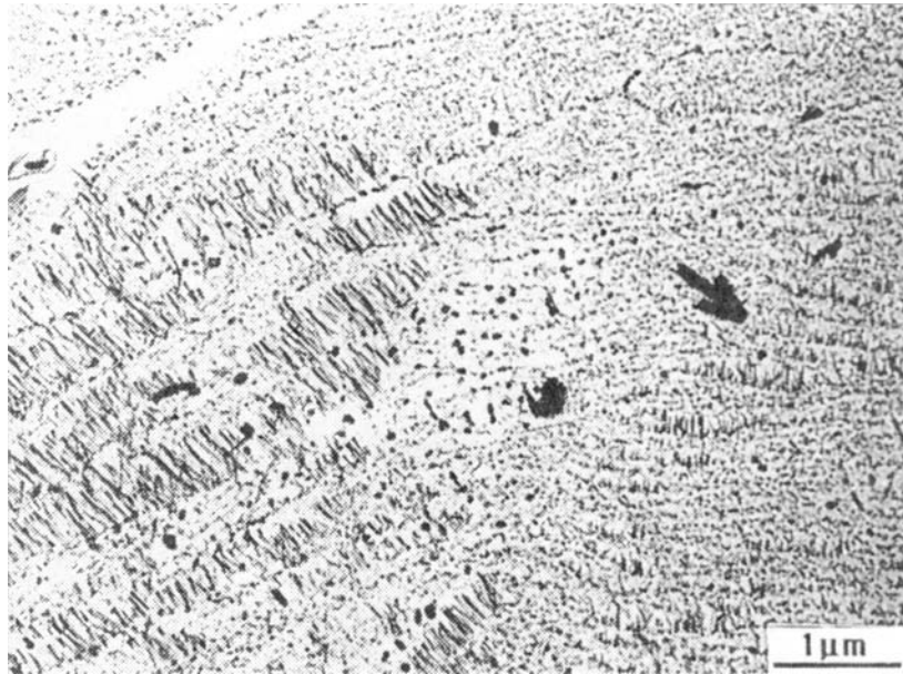
Figure 4 Fibrous morphology of microalloy precipitates in ferrite. (From Ref. 113.)
