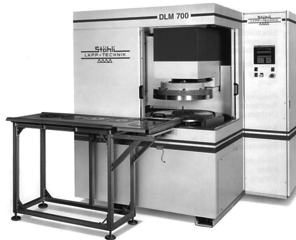
FIGURE 16.75 Stahli DLM 700 double-sided fine grinder.
