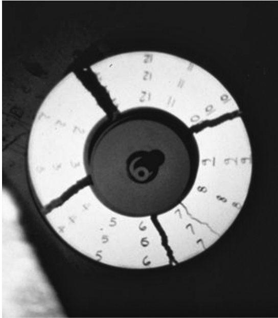
FIGURE 4.9 Solid wheel failure 90 m/s. Monolithic alox body.
