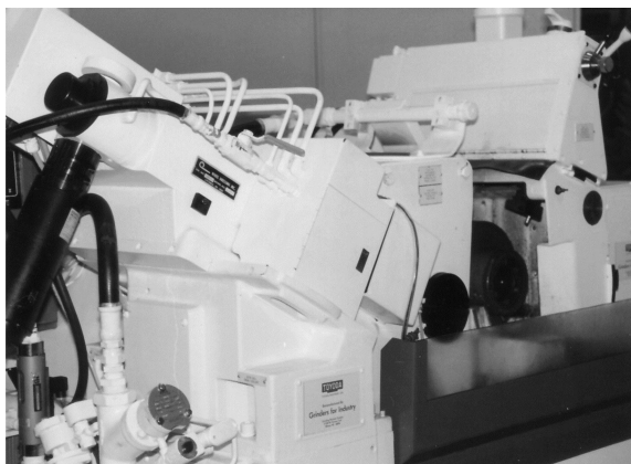
FIGURE 15.62 Rebuilt Cincinnati 220-8 centerless grinder with servo-driven plunge rotary diamond dressing.
