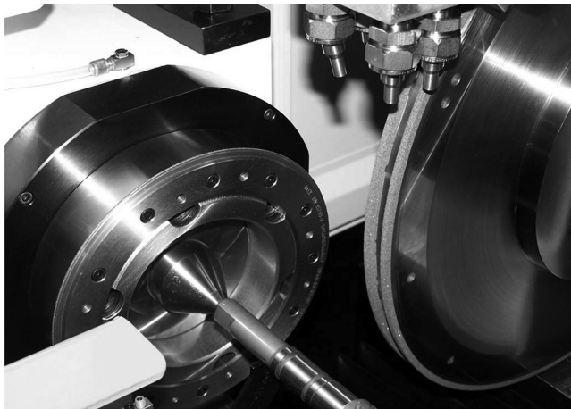
FIGURE 7.27 Work head mounted dresser on a Weldon peel grinder.
