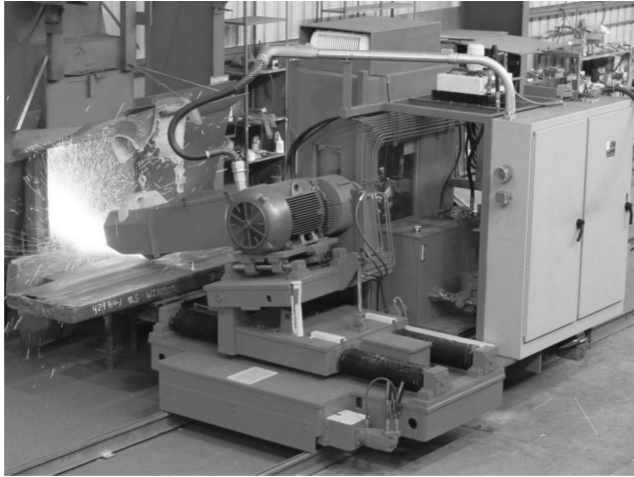
FIGURE 5.11 Billet grinder. (Courtesy of MidWest Machines.)
