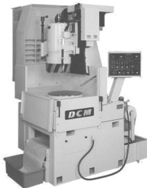
DCM tech IG 280M rotary surface grinder with segmented wheel detail
