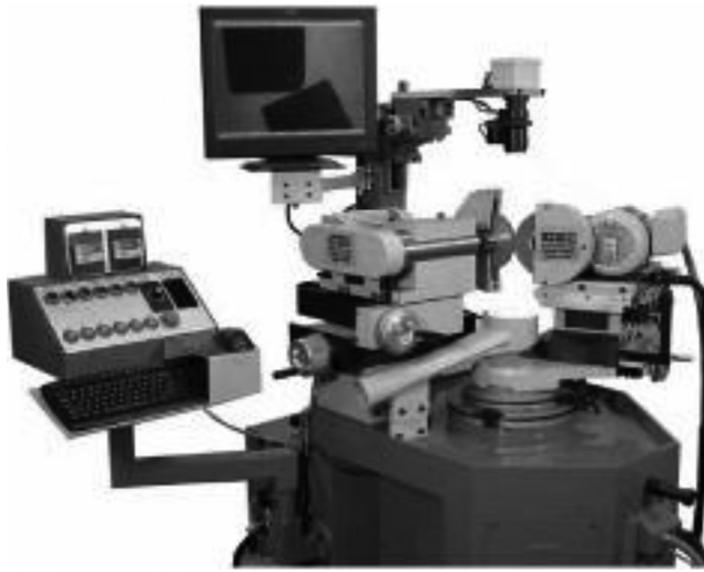
FIGURE 7.44 Offline dresser for resin, hybrid, and dense superabrasive wheels.
