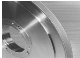
CBN wheel for rough grinding of crankshaft to replace turn broaching
