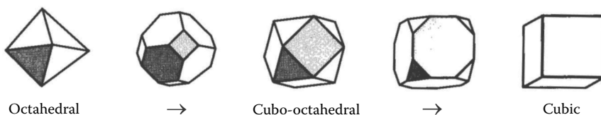
FIGURE 5.22 Growth morphologies of diamond.
