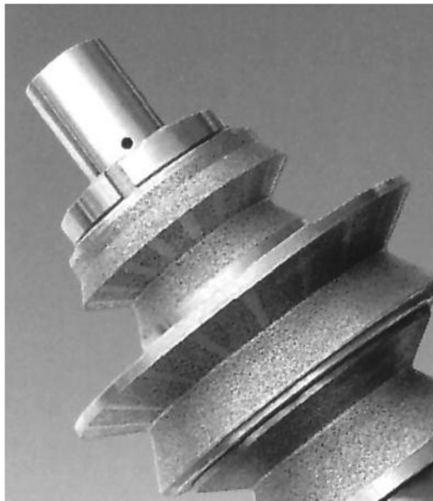
FIGURE 7.35 Diamond free areas on shoulder of reverse-plated roll.
