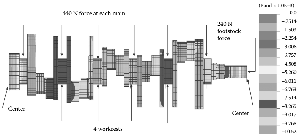
FIGURE 17.39 FEA analysis of the effect of forces on the crankshaft during grinding.
