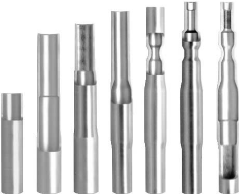
Figure 16 Process Chain Illustrated by Part Stages in Car Transmission Shaft Production. (Courtesy FELSS, Königsbach-Stein, Germany)
