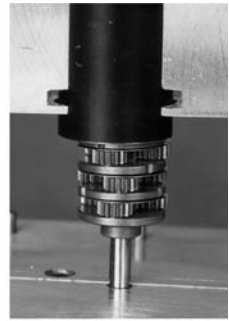
joining of gearwheel housing
