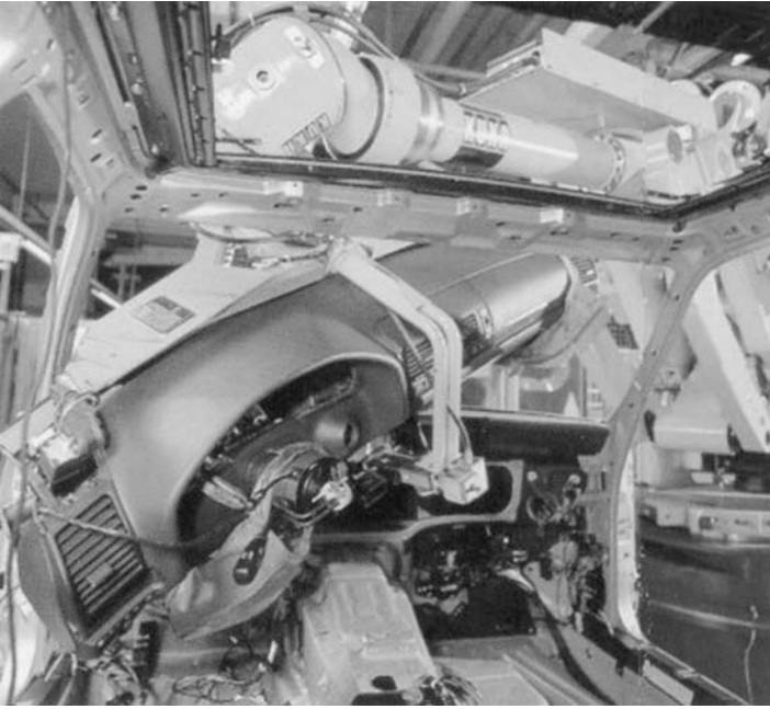
Figure 36 Assembly of Driver Control Instruments. (Source: KUKA Roboter GmbH)
