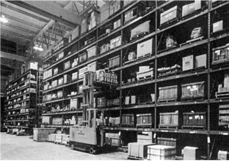
Figure 18 Single-deep Selective Rack.
