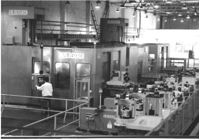
Figure 13 FMS for Oil Well Drill Production.
