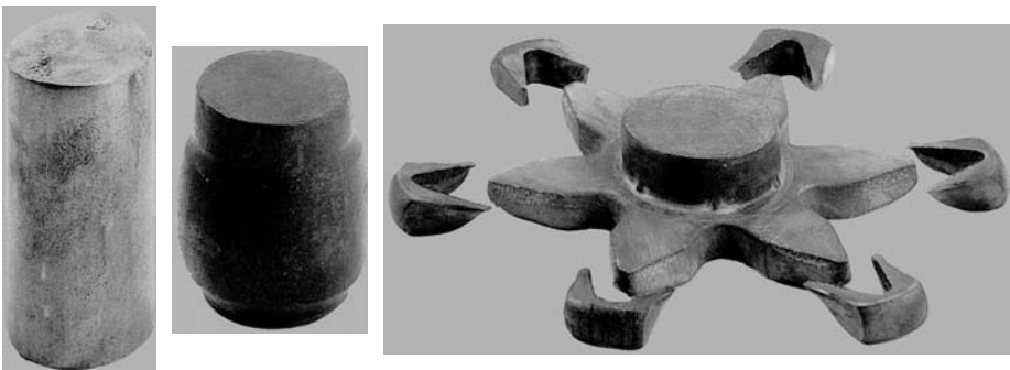
Figure 23 Hot Extrusion of Field Spiders. (From Körner and Knödler 1992)
