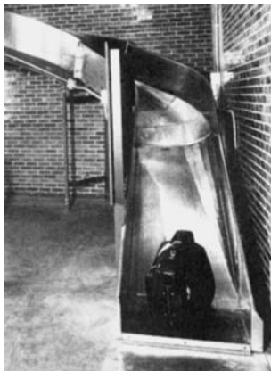
Figure 8 Chute Conveyors. (Courtesy of Standard Conveyor Company)
