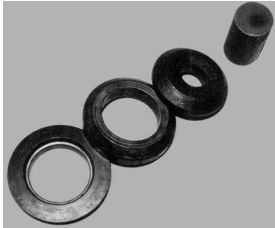
Figure 25 Axial Die Rolling of Car Bevel Gears. (From firm prospectus, courtesy SMS Eumuco, Leverkusen, Germany)
