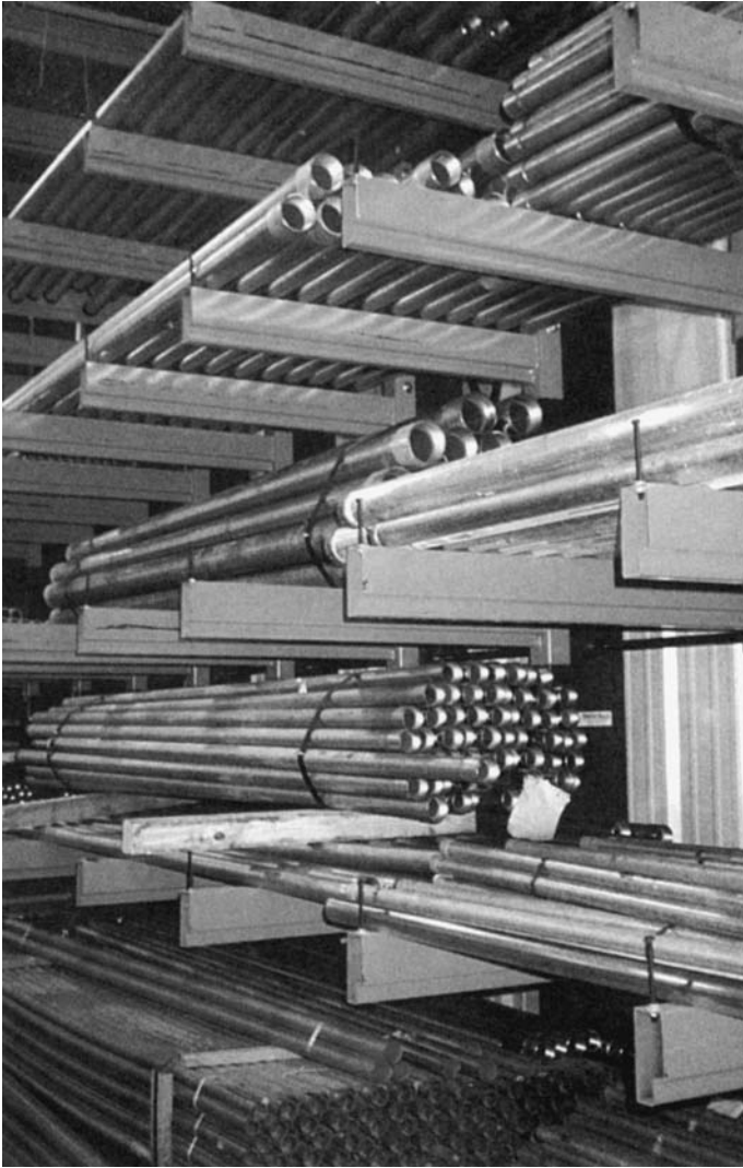
Figure 20 Cantilever Rack. (Courtesy of Jervis B. Webb Co.)
