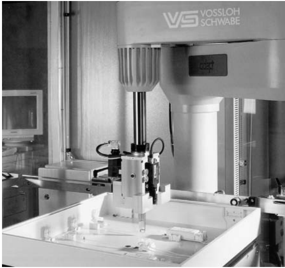
Figure 43 Assembly Cell for Automatic Wiring of Luminaires. (Source: Vossloh Schwabe GmbH)
