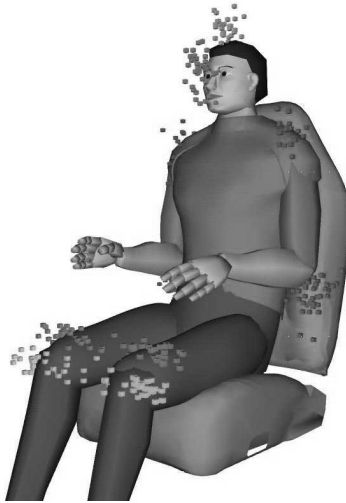
Figure 4 The Anthropometric Landmark Data from Multiple Subjects Is Displayed in the Form of Data Clouds. The simultaneous view of the data allows for rapid assessment of control location and adjustment questions. (Courtesy Dr. Jerry Duncan, John Deere Corporation)
