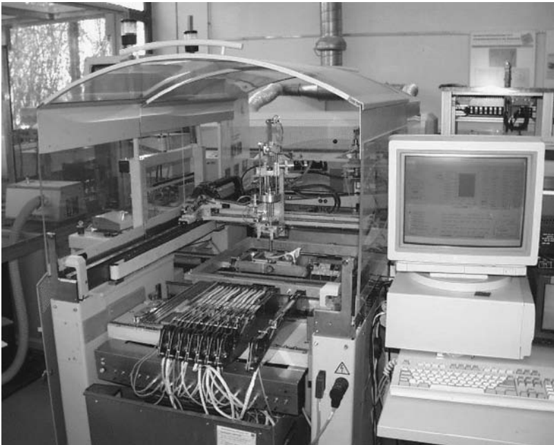
Figure 45 Prototypical Realization of MID Placement System for 3D assembly. (From Feldmann et al. 1998)
