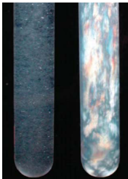
Figure 2.20 Aqueous 0.53% (w/v) suspensions of CNs observed between crossed polarizers after production by HCl-catalyzed hydrolysis (a), and after their oxidation via TEMPO-mediated reactions (b). Reproduced from [110], copyright 2006 © permission from Springer.
