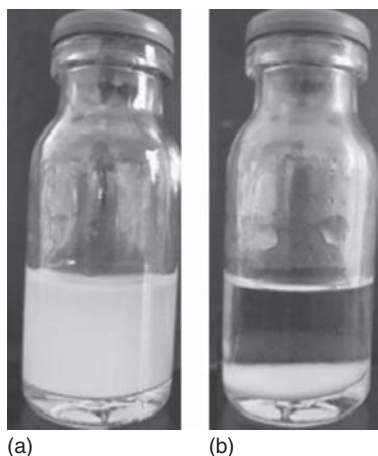
Figure 2.34 Dispersion of starch nanocrystals in water (a) settled 0 min and (b) settled 30 min. Reproduced from [152], copyright 2012 © permission from Elsevier.
