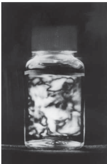
Figure 2.21 Polarized optical micrographs of the silylated CN suspension in THF. Reproduced from [106], copyright 2002 © permission from Elsevier.
