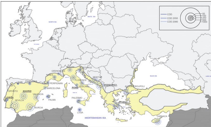
Fig. 4.8 Map of Southern Europe with selected locations and their cooling degree days, CDD (27 °C), for current scenario and H2050 future scenario, over EEA delimitation
