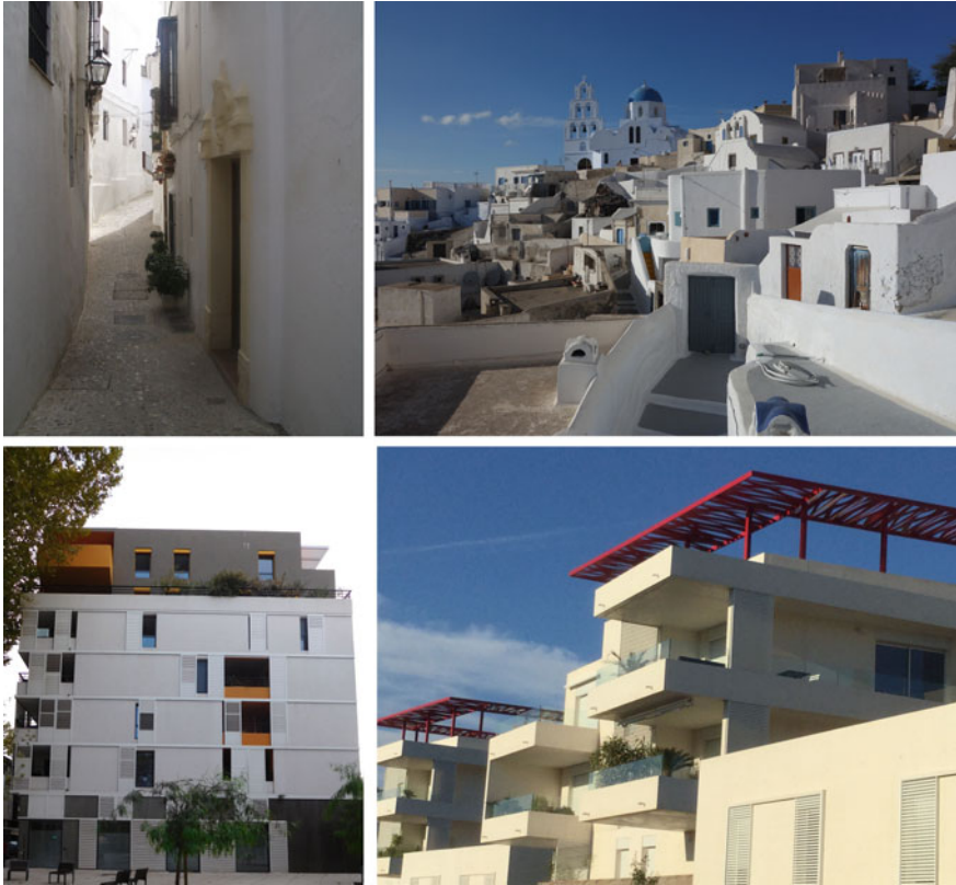
Fig. 8.20 Examples of architecture that incorporates materials with high reflectance (albedo), both in traditional architecture (Andalusian street in Spain, and Santorini in Greece), and in new residential buildings (Montpellier, France)
