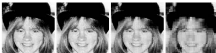
Original 'Jo'. 1% error, using 5% error, using 10% error, using ( 128 \times 128 ) 55% of coefficients. 12% of coefficients. 3% of coefficients.
