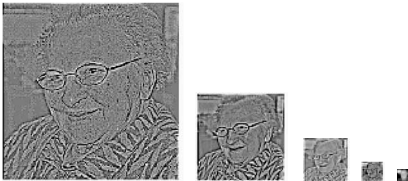
Figure 15.38 The Laplacian pyramid of differences L_k = g_k - \text{EXPAND}(g_{k+1}) . This sequence is the encoded version of the original: (L_4, L_3, L_2, L_1, L_0) .
