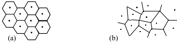
Figure 11.13 Partitions of the plane obtained by inserting decision boundary lines where the points m_i are (a) centres of a honeycomb partition (thereby recovering the hexagonal edges), (b) randomly scattered points. In either case, a boundary edge is the perpendicular bisector of the line joining the points m_i, m_j that define it.
