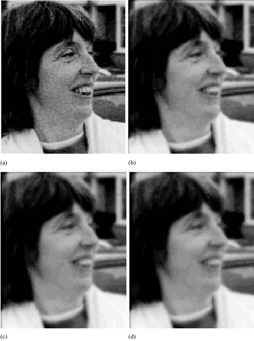
Figure 15.20 (a) 128 \times 128 image (slightly cropped), undersampled, and therefore containing zigzag edges and other signs of 'pixillation', (b), (c), (d) smoothing with Butterworth filter of order 1 and cutoff 20, using respective sizes 3, 5, 7 as recorded in Example 15.27. The smoothing even by size 3 gives a dramatic improvement in quality at the expense of a slight blur. Perhaps only the mouth benefits by going up to size 7.
