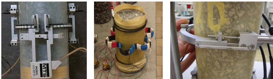
Figure 4: Chain-extensometer (left), steel spring device (middle), LVDT device (right) (Kappl, 2007)
