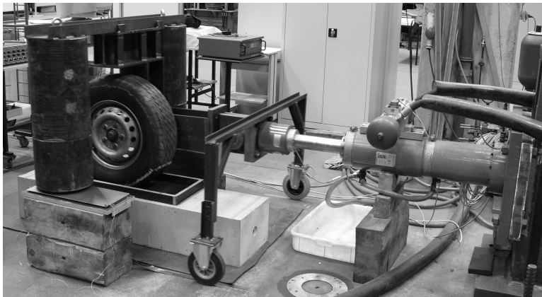
Figure 11. Penetration-test of sodium chloride solution due to over rolling movements of a tire
