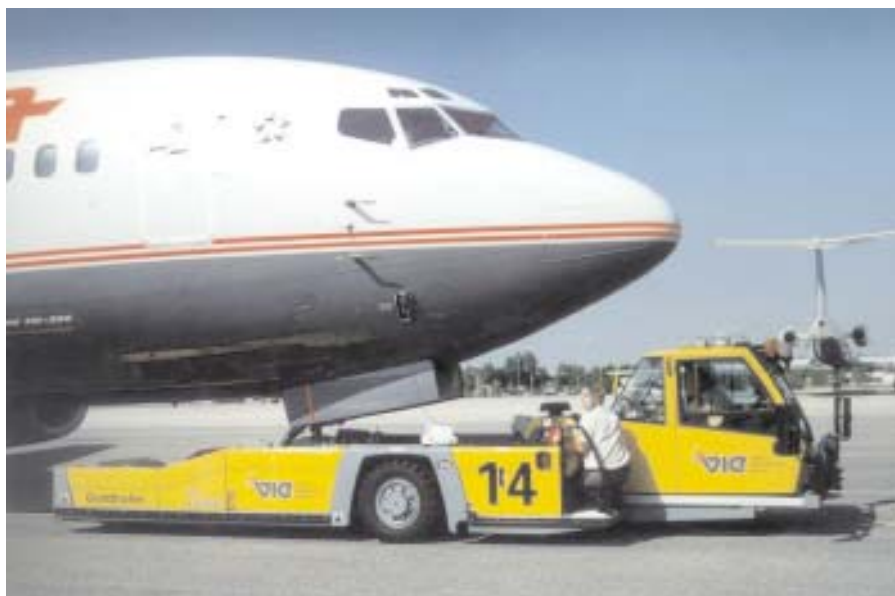
Figure 1. TLTV with the nose gear of an aircraft to be towed captured in the nose gear cradle (photograph courtesy of Goldhofer Airport Technology).
