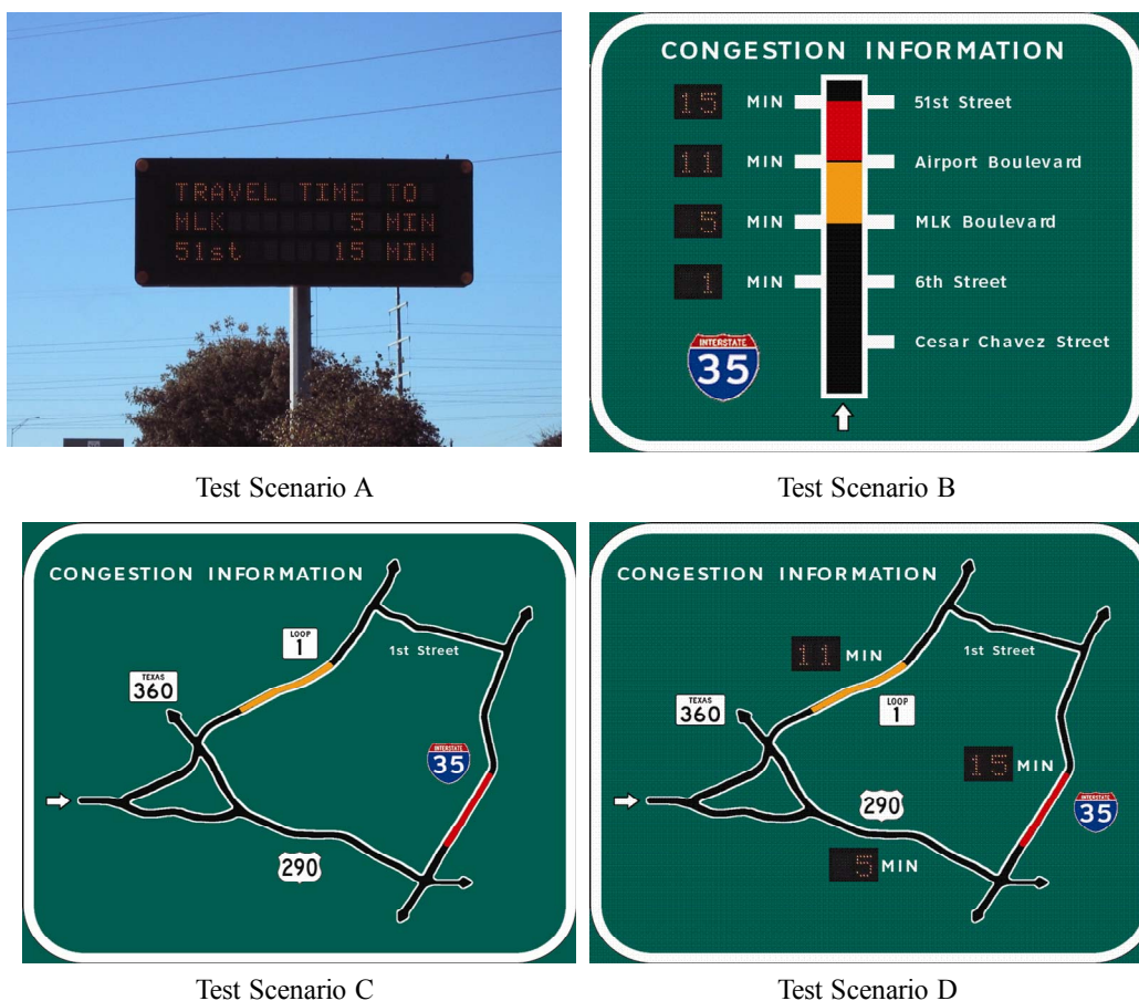
FIGURE 2 Schematic Sketch of the DMS and GRIPs for Test Scenarios A to D
