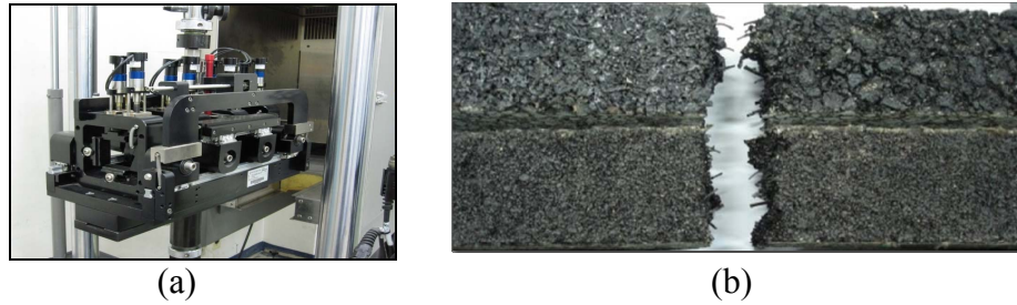
Figure 6. (a) Four-point bending beam fixture and (b) Fiber-reinforced specimen after failure
