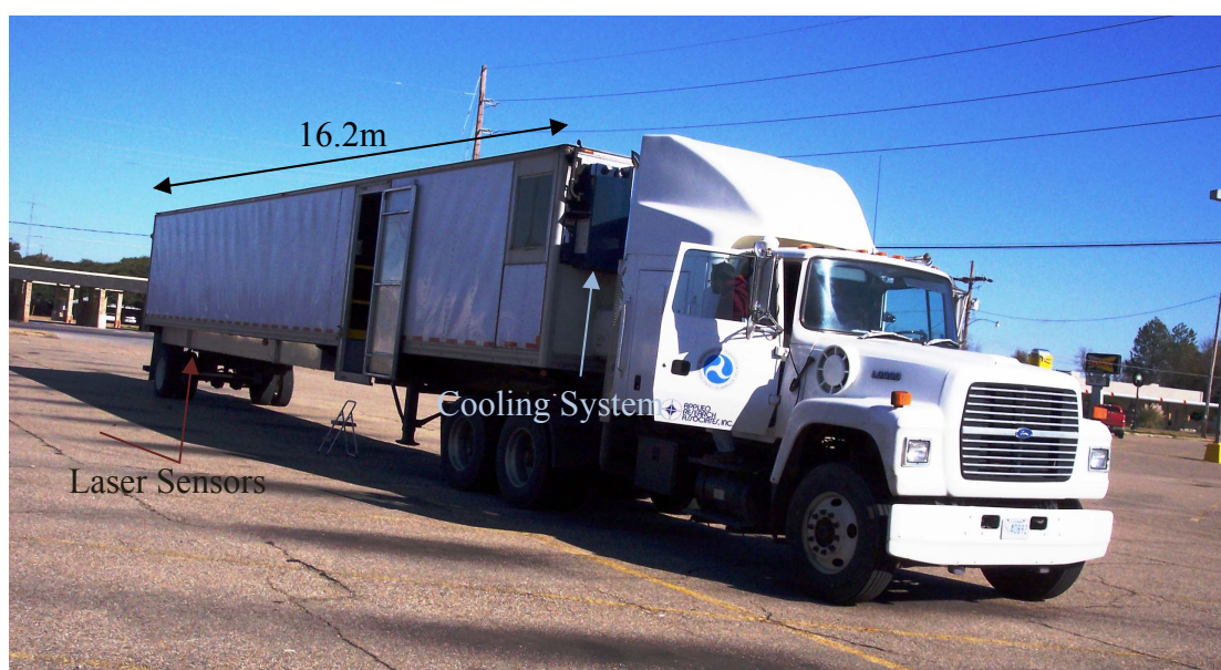
Figure 1. General Overview of the Rolling Wheel Deflection System
