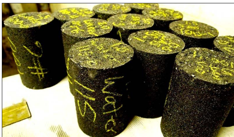
Figure 3. Warm asphalt mixture produced using the water foaming method
