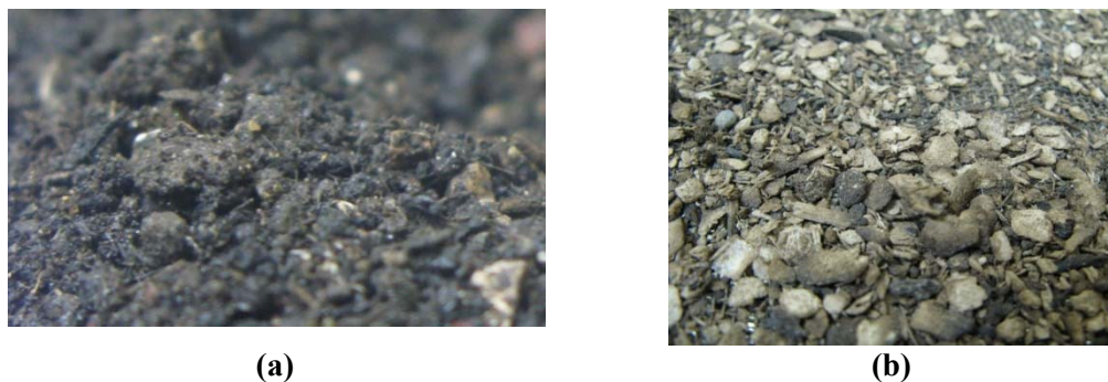
Figure 1. Shingles (a) before and (b) after the process of extraction and recovery
