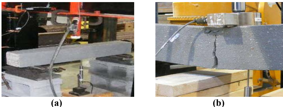
Figure 2. (a) Flexural fatigue test system, (b) piston applying force to load cell
