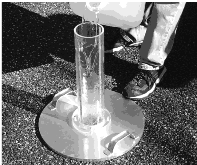
Figure 6 – Field test apparatus using falling head permeability test
