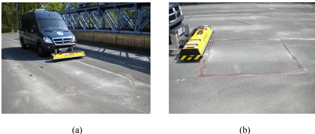
Figure 3. APE system scanning embedded in-pavement (a) diamond shaped loop wire seen as adhesive filled saw cut marks in the pavement surface in the foreground of the photograph and (b) square shaped loop wire.
