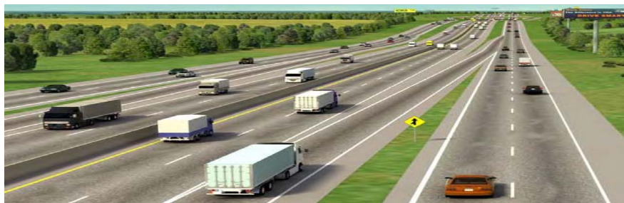
a) Proposed truck-only lane slip ramp configuration
