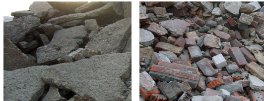
Figure 1. Original concrete rubble (left) and masonry rubble (right).
