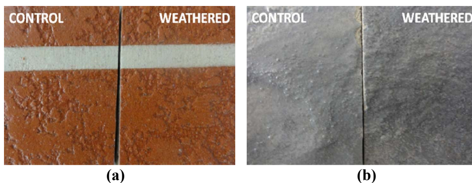
Figure 5. UV-exposure results (a) DCO-brick control vs. weathered brick, (b) DCO-stone control vs. weathered stone
