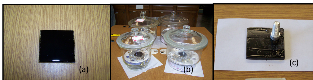
Figure 1. Sample Preparations for Dry Cohesive Strength: (a) Asphalt Samples, (b) Asphalt Samples in Desiccators, and (c) Pull-Stub Samples.
