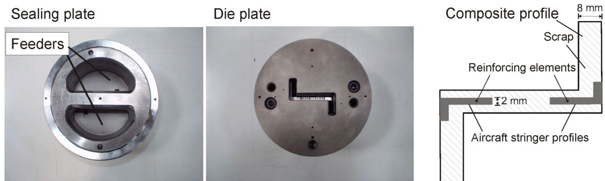
Figure 2: Modular die concept of the tool design and extruded Z-profile cross section
