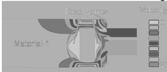
Figure 2: Example of dead zones in the material flow for the initial die design
