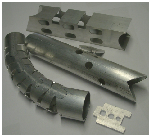
Fig. 5: Experimental samples of reinforced and unreinforced profiles processed with CO 2 laser.
