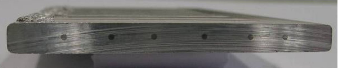
Fig. 3: Flat profiles with reinforcement elements; 56 x 5 millimeters
