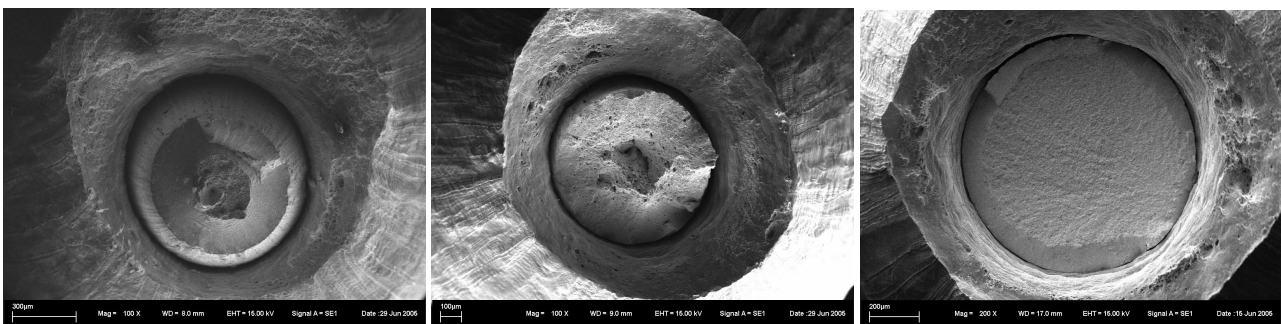
Fig. 6: SEM micrographs of fractured tensile specimens for the sample states S1 (left), N1 (centre) and C1 (right)
