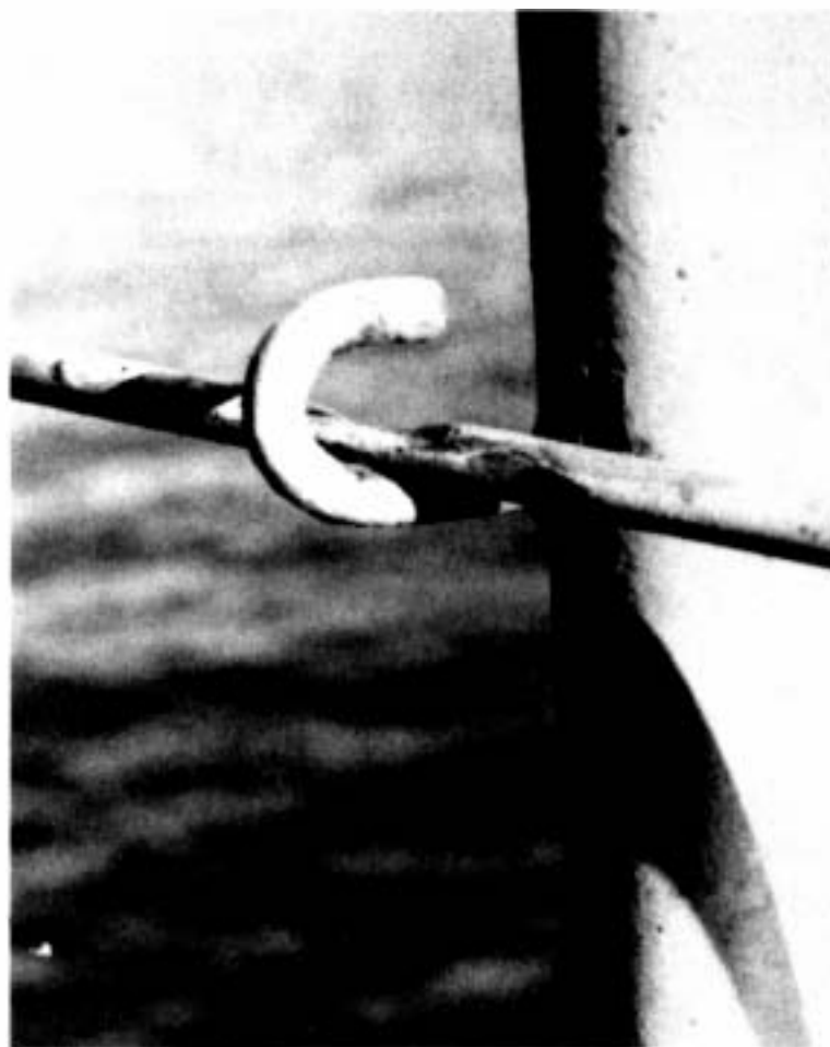
Figure 4-52 Worn Nonmetallic Lifeline
