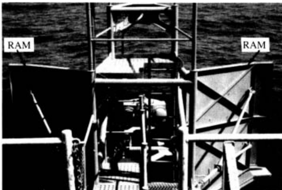
Figure 4-22(b) RAM Barriers Protecting Aircraft Carrier ECM System
