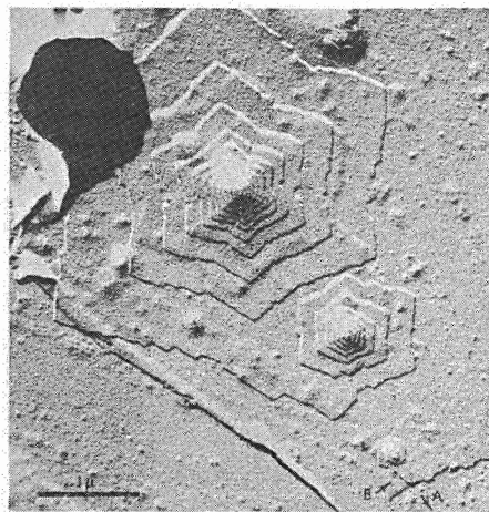
Fig. 15.18: Spiral growth on a polyoxymethylene crystal due to two screw dislocations of opposite nature.
