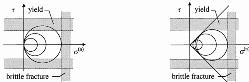
Fig. 22.11: Mohr's circles showing competition between flow and fracture in plane stress (left) and plane strain (right).
