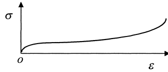
Fig. 23.2: Typical stress-strain curve for rubber.
