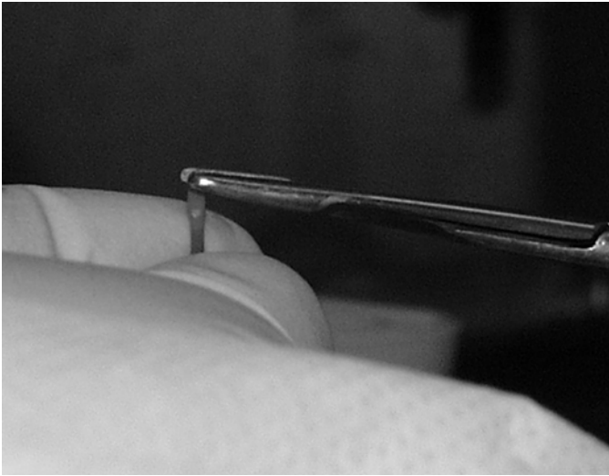
Fig. 2. Heat-sealing the end of cell-loaded fiber using needle holder.
