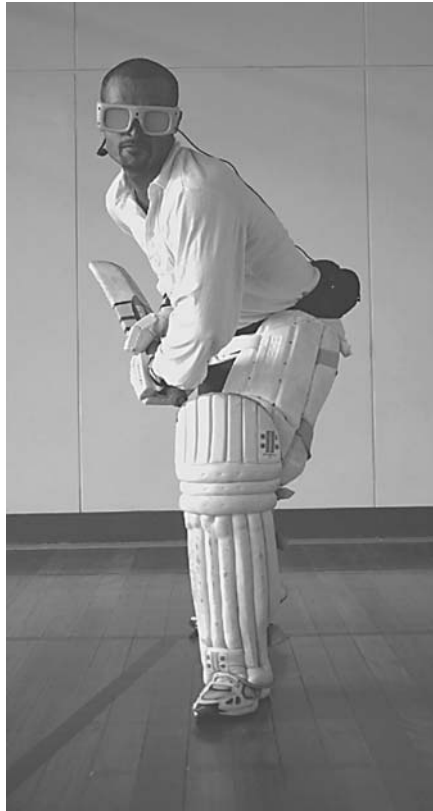
Figure 11.3 Liquid crystal goggles worn by a batsman while playing a stroke. The goggles are connected to a lightweight radio transmitter strapped to the player's waist. Occlusion of vision can be triggered through an infrared controller remote to the batsman. Reproduced by permission of Chérie Harris
