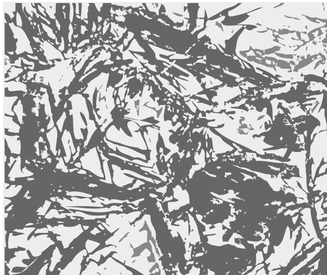
FIGURE 4-15 Microstructure of Martensite
