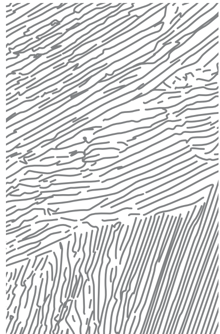
FIGURE 4-13 Microstructure of Pearlite
