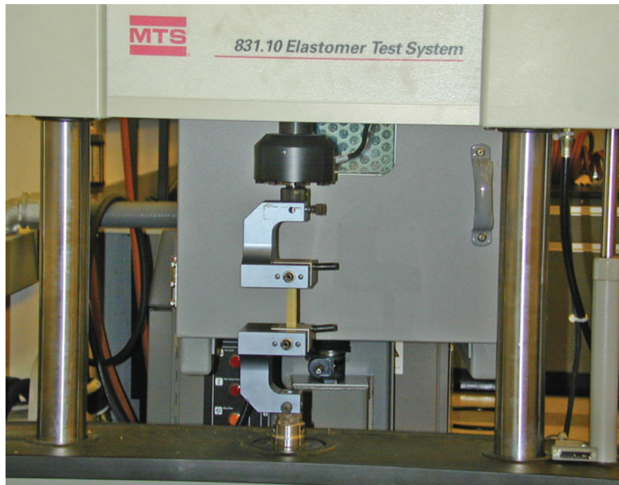
FIGURE 3-2 Photograph of a Tensile Test on a Kevlar®-Epoxy Composite
