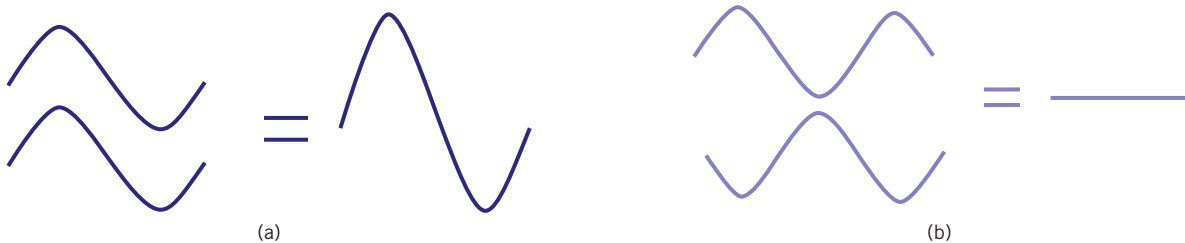
FIGURE 2-10 Interference Patterns for X-rays: (a) Constructive Interference; (b) Destructive Interference
