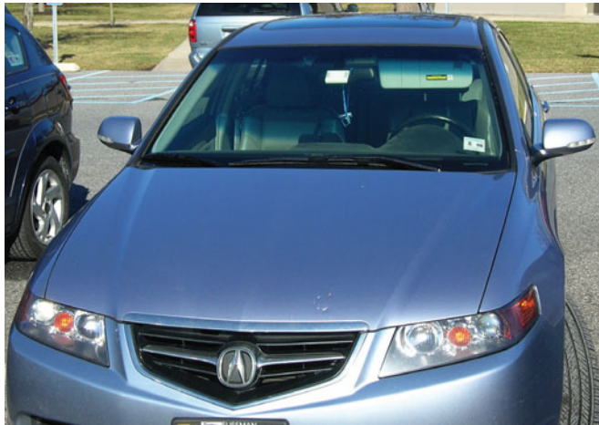
FIGURE 1-3 Curved and Tinted Windshield on a Modern Acura
