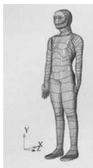
Fig. 1. Panel distribution representing a standing configuration.
