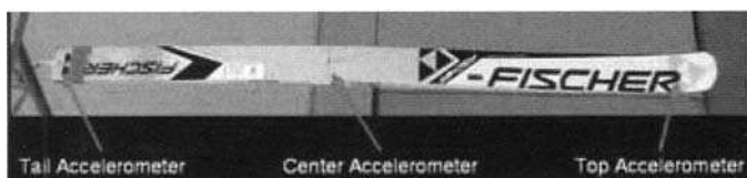
Fig.2. The jump ski used in the impulse response experiment in this study
