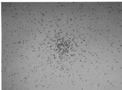
Fig. 6. An example of the gathering of Euglena to the laser beam at the population density of culture medium: 190 \text{ cells/mm}^3 , taken after 90 minutes laser irradiation
