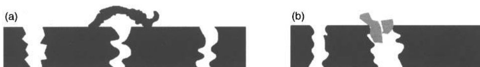
Figure 6.15. Schematic diagrams showing (a) bridging mechanism and (b) occluded pore when particles are trapped within a filter. Used with permission from Pall Corporation.
