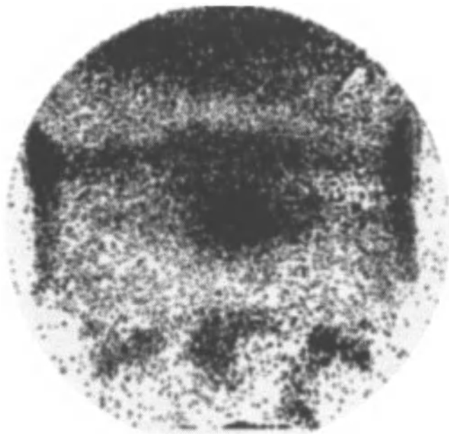
Figure 2.15. Light point defect distribution on a bare silicon wafer after dipping in Cu-spiked HF followed by a clean APM step [34]. Reproduced with permission of ECS – The Electrochemical Society from Knotter, D. M., Gendt, S., Mertens, P. W., and Heyns., M. M., Journal of the Electrochemical Society .
