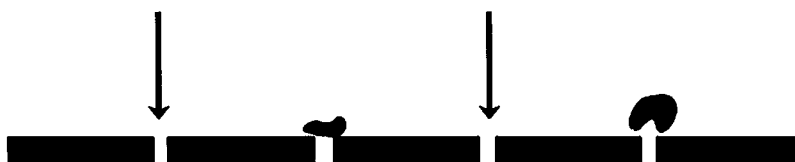
Figure 6.14. Schematic of the sieving mechanism of a filter. Used with permission from Pall Corporation.
