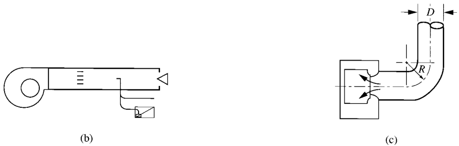
FIGURE 20.5 Inlet system effect: (a) inlet system effect on the \Delta p_t - \dot{V} diagram; (b) fan test unit at laboratory; (c) round elbow before fan inlet.
