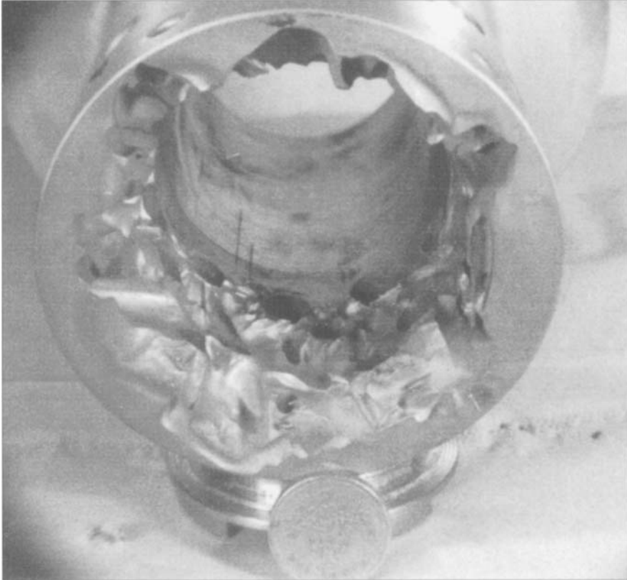
Fig. 2.6 Erosion by hard particles in a high-velocity fluid stream
