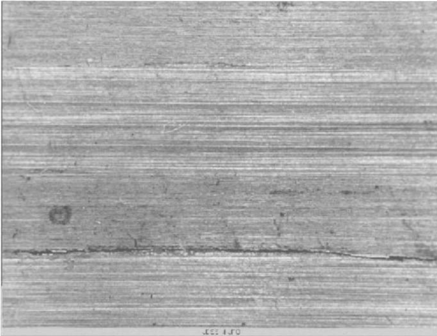
Fig. 2.2 Abrasive wear from hard particles trapped between moving surfaces
