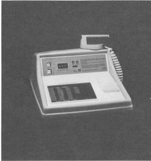
FIGURE 9-25. Examples of external noninvasive programmers for implanted permant generators. A, Medtronic 9701 (desk-top) and 9700 (hand-held) Spectrax programmer. B, Medtronic 9701A (desk-top) programmer for DDD, DVI, and VVI generators. C, Cordis 256A (desk-top) interactive programmer for all available Cordis generators. D, Cordis 255A (hand-held) programmer, which incorporates many of the features of the 256A device. (Courtesy of Medtronic and Cordis Corporation.)
