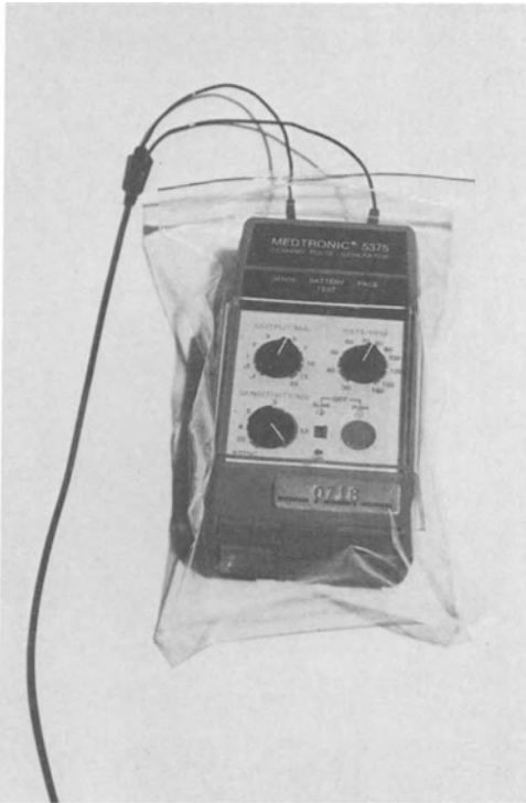
FIGURE 9-17. Insulation of temporary pacing generator. To avoid the hazard stray electrical currents gaining access to the exposed lead terminals, the entire assembly should be surrounded by a nonconductive material (e.g., enclosed in a plastic bag or glove).
