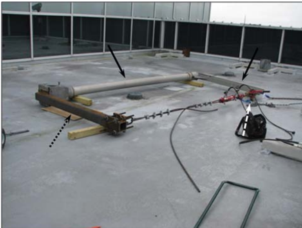
Figure 9. Load testing of a davit arm. The black arrows indicate the davit arm. The dotted black arrow points to the reaction test rig. The test is self-contained, and the arm is reacting against itself. The dashed white arrow indicates the hydraulic jack.
