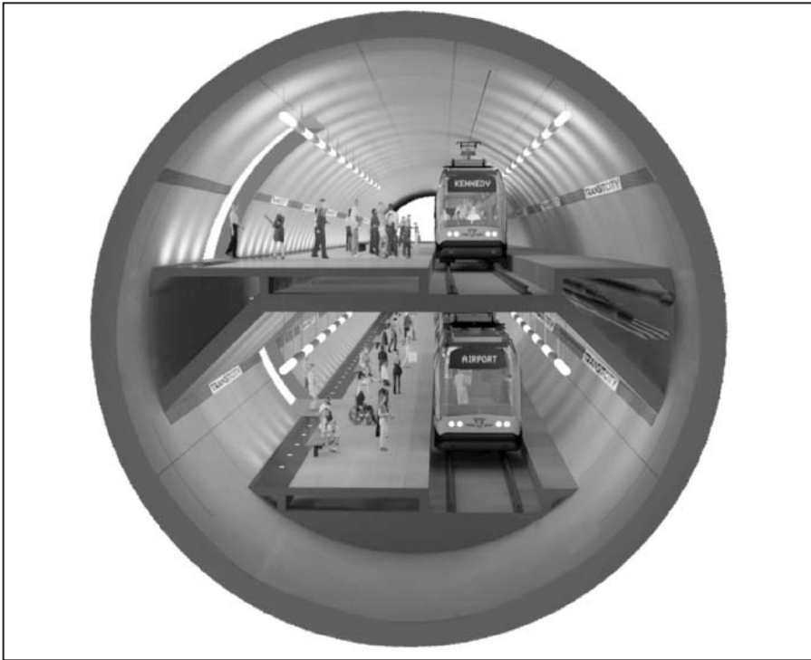
Figure 5. Single tube station platform
