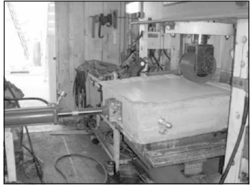
Figure 12. PVC liner testing
