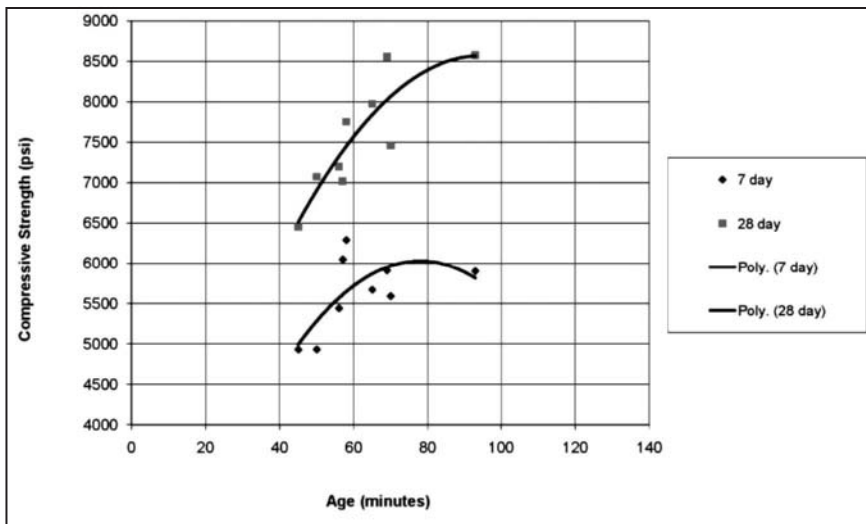
Figure 6. Shotcrete compressive strength versus age of mix
