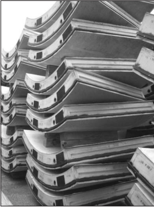
Figure 1. PVC lined segments with flaps
