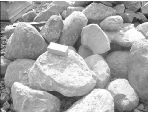
Figure 3. Boulder and cobbles excavated in soft-ground zone
