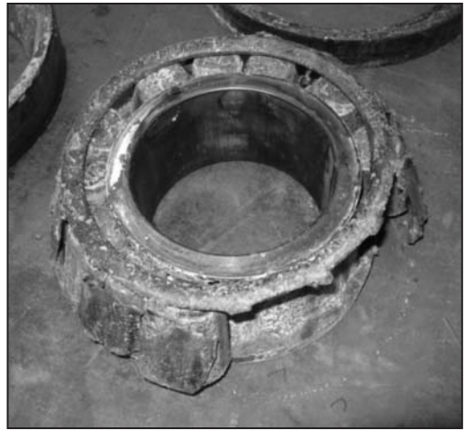
Figure 2. Failed cutter bearing
