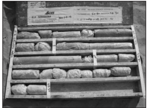
Figure 5. Core box containing plastic wrapped core from T-03 borehole, SB-117
