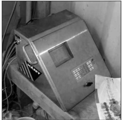
Figure 9. Automatic data recording system (Hany Computer)
