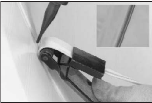
Figure 5. Hot air welding 1" weld strip using weld strip roller
