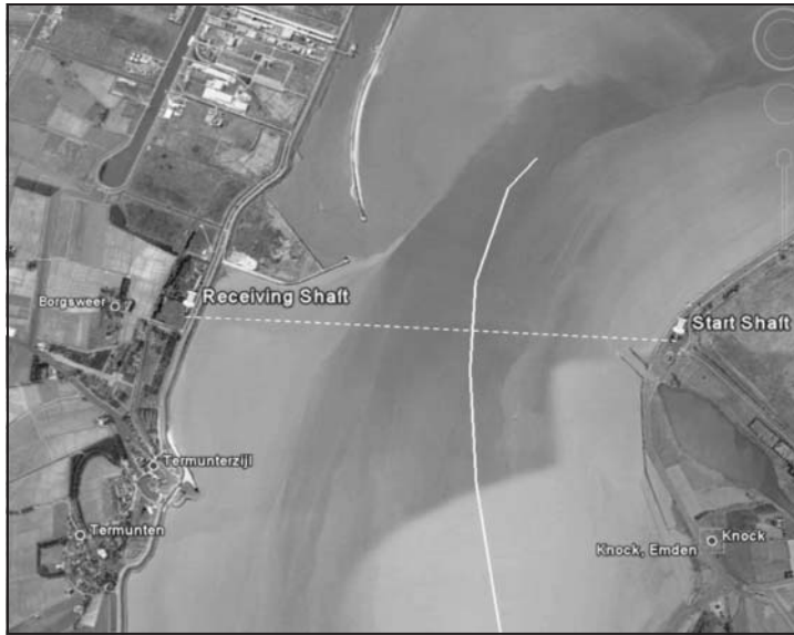
Figure 1. Overview of start shaft and receiving shaft
