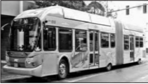
Figure 10. BRT vehicles with two driver-side doors
