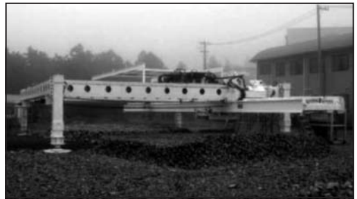
Photo 5. Underwater crushed rock leveling robot
