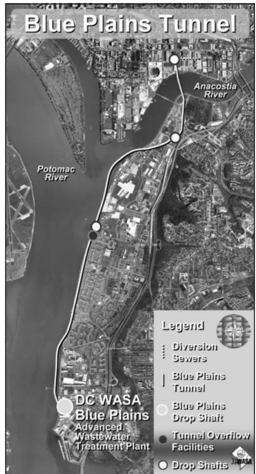
Figure 3. Blue Plains tunnel alignment
