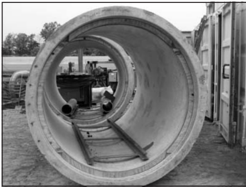
Figure 7. Photo of reinforced concrete pipe showing wood packers
