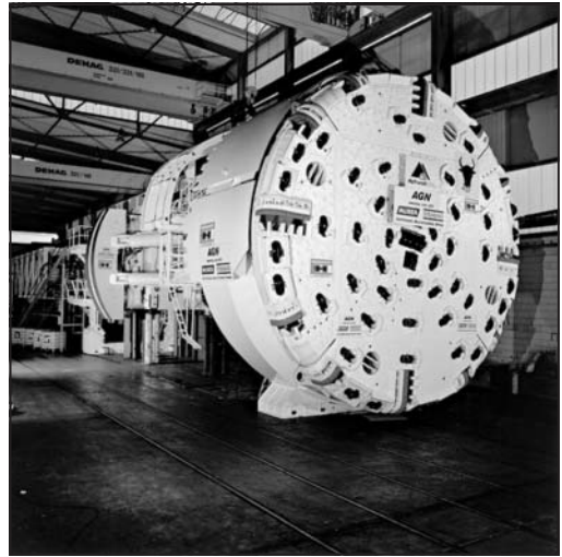
Figure 5. Hard rock gripper TBM at Amsteg
