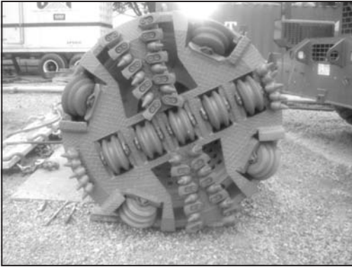
Figure 4. MTBM cutting head, fitted with drag teeth, bullet teeth, and roller cutters
