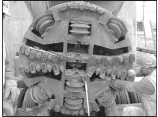
Figure 5. Cutter head after first run showing wear on teeth
