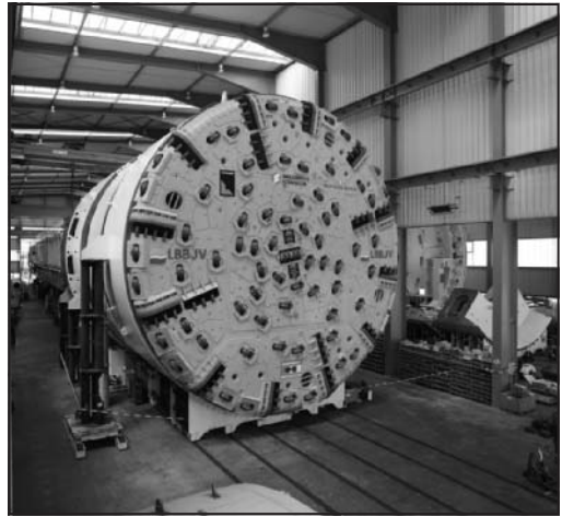
Figure 4. Cutterhead of double shielded hard rock TBM Ø12.34 m for the north bound tunnel in Brisbane
