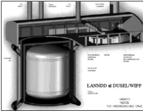
Figure 3. LAr and neutrino nucleon and nuclear decay detector LANNDd concept (Source: Cline, 2001)
