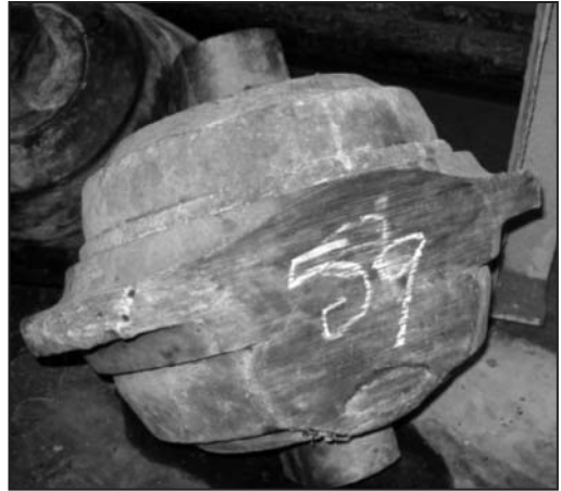
Figure 3. Non-rotating cutter damage
