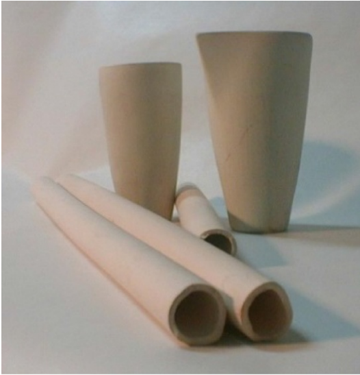
Fig. 7.8 Al-sludge-based bodies processed by extrusion and slip casting (Ribeiro et al., 2004a).
