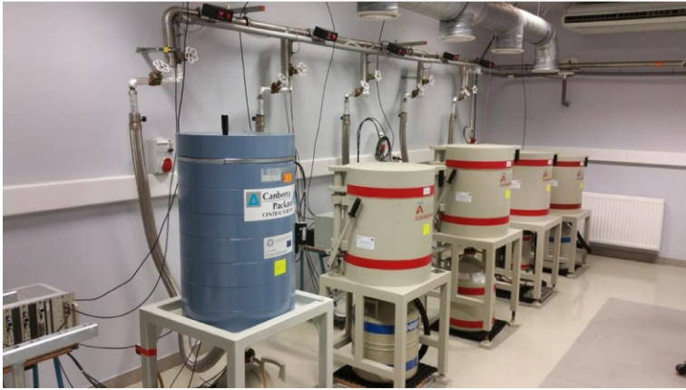
Fig. 5.11 High-resolution gamma spectrometry laboratory in the Silesian Centre for Environmental Radioactivity, Central Mining Institute, Katowice, Poland.
