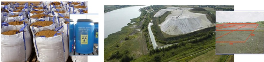
Fig. 5.7 Types of NORM residues created on regular basis as a result of a well specified technological process (left), or already accumulated (e.g., phosphogypsum, right) could be potential raw materials for the construction material industry.
