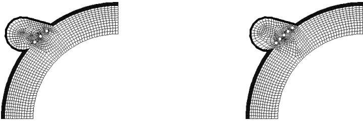
Fig. 9. Deformed mesh for steady configuration with stents: 3 stents (left) and 5 stents (right).
