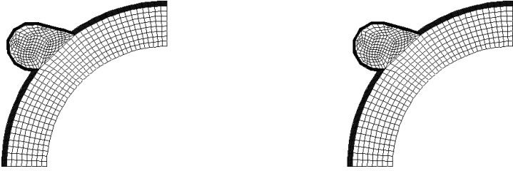
Fig. 8. Deformed mesh for steady configuration without stents, with elastic wall (left). Mesh for rigid wall (right).
