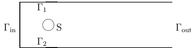
FIGURE 11. Configuration of the benchmark problem ‘viscous flow around a circular cylinder’ with outlets \Gamma_{1,2} for boundary control by pressure variation.
