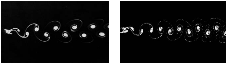
FIGURE 1. Experiment (source: Van Dyke’s ‘Album of Fluid Motion’) vs. numerical simulation (source: ‘Virtual Album of Fluid Motion’) for flow around a cylinder.
