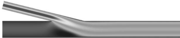
FIGURE 2. Configuration of flow through a bifurcating pipe.
