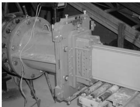
Fig. 20 Hydraulically optimized combination pressure head and die assembly for facing tiles
