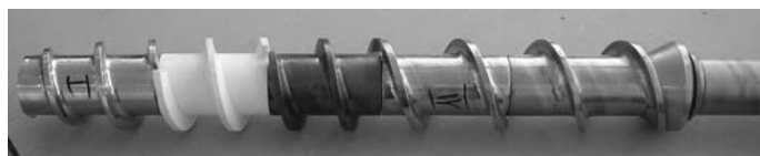
Fig. 34 Auger segments in various materials for extruders in technical ceramics
