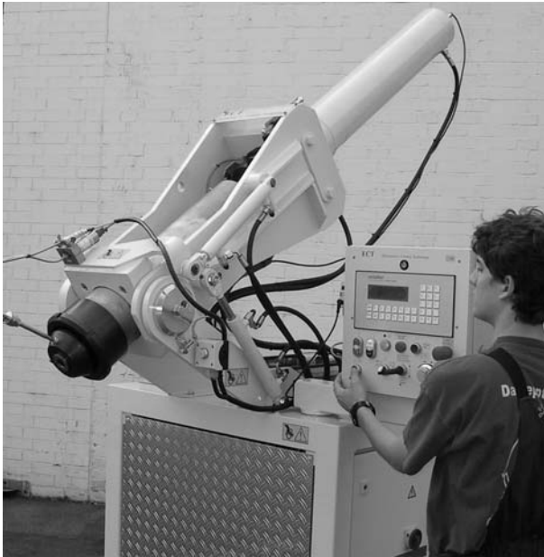
Fig. 5 140 mm piston extruder with tilting press frame
