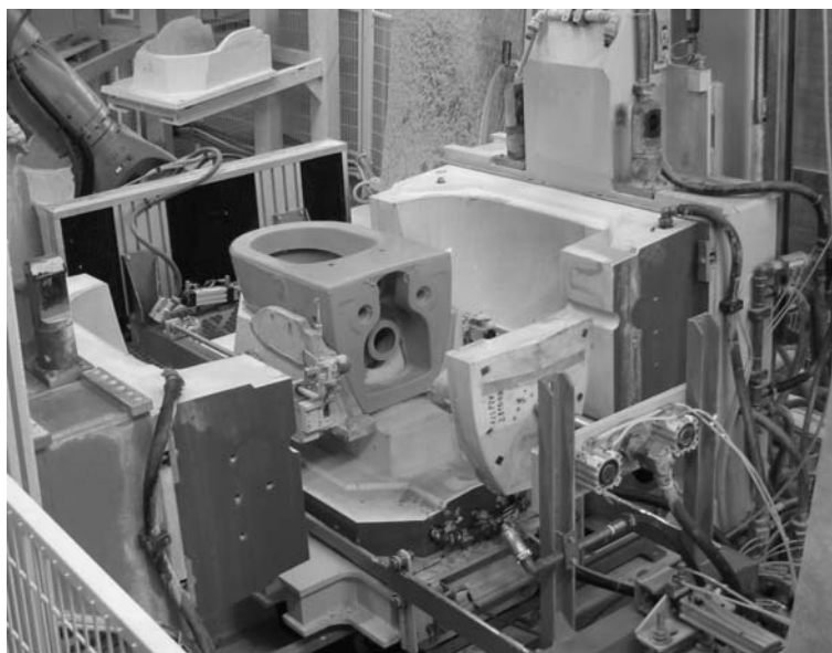
Fig. 14 High pressure casting machine
