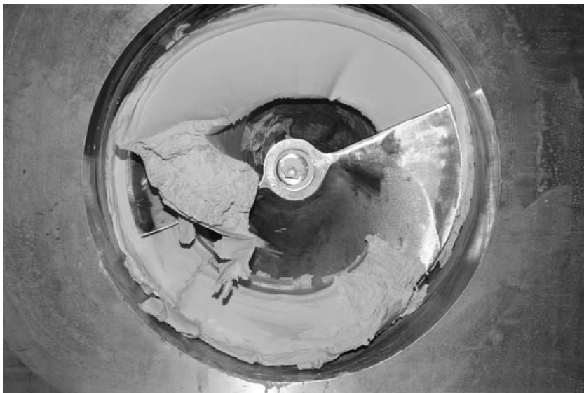
Fig. 9 Mass flow at the top auger
