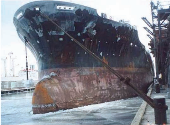
Fig. 4-17. Vessel moored alongside in ice of moderate thickness Source: Photo reproduced courtesy of Appledore Marine Engineering
