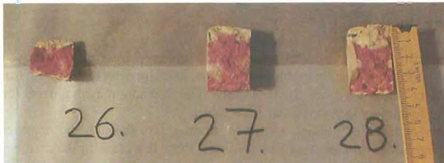
Fig. 3-8: Determination of carbonation depth with Phenolphthalein, (Vollrath, Tathoff 1990, [152])
