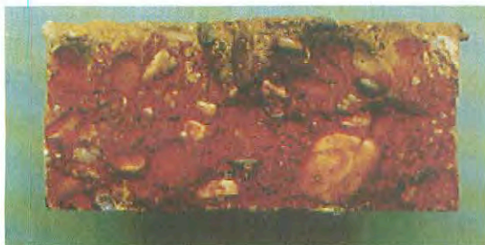
Fig. 3-9: Qualitative determination of Chloride ingress, (Vollrath, Tathoff 1990, [152])
