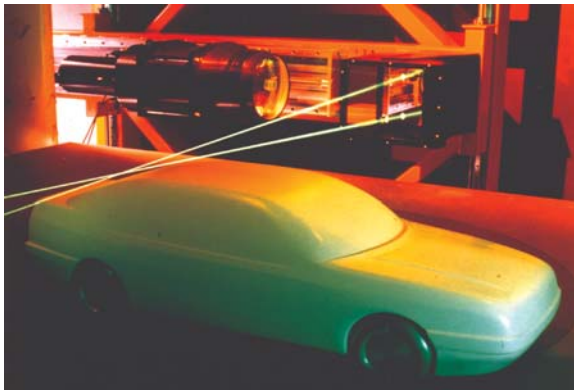
Fig. 1.6 Flow investigation with the aid of a laser Doppler anemometer
