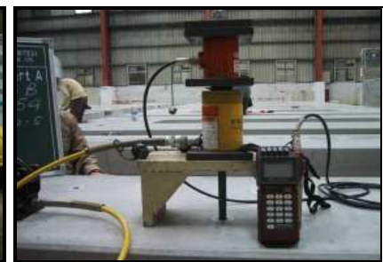
Fig.6 Pulling test of plug A & C
