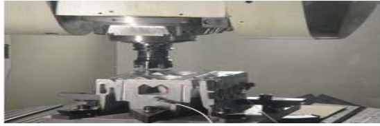
Fig.4 Vibration Monitoring of Machining Process
