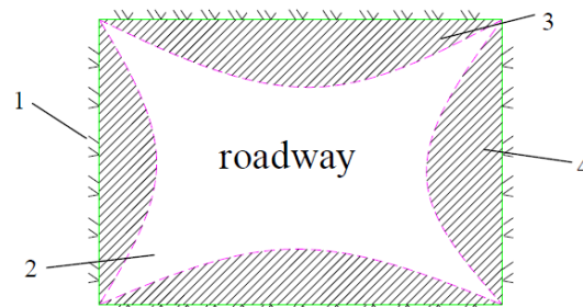
Fig. 2 The surrounding rock deformation of the roadway in high stress
