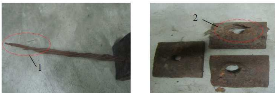
(a) Damaged cable
