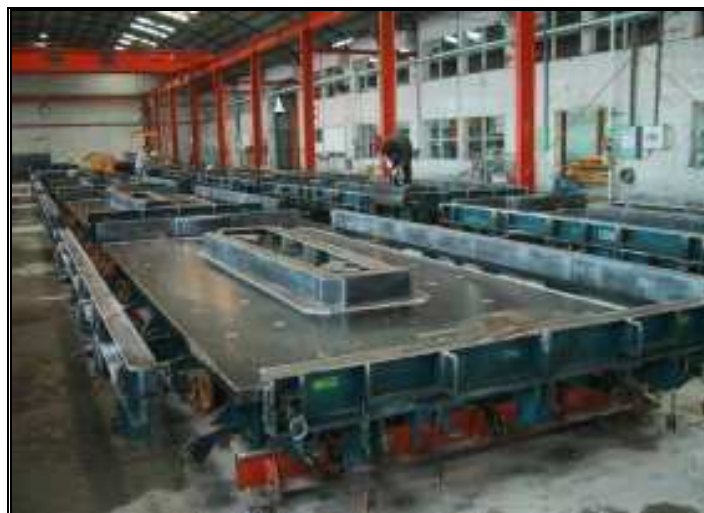
Fig. 3 Molds for slab tracks
