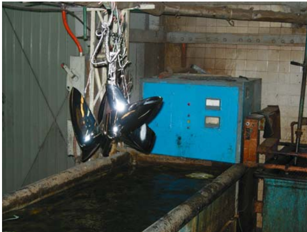
Fig. 3. Metal pieces after treatment in galvanising bath
