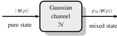
Fig. 11.23 A Gaussian state |\psi(p)\rangle is sent through an additive-noise Gaussian channel. At the output the state is still Gaussian but it becomes a mixed state \rho_{\mathcal{N}}(\psi(p))
