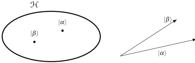
Fig. 7.3 Two distinct coherent states are never orthogonal: \langle \alpha | \beta \rangle \neq 0
