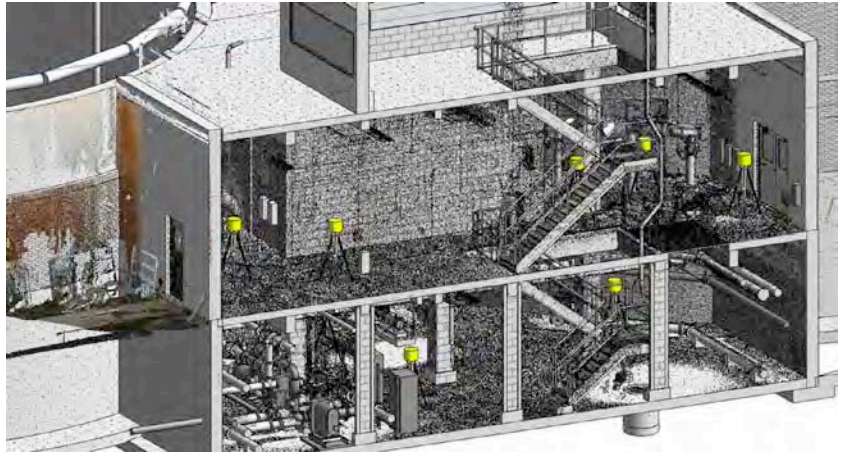
FIGURE 21.2 Creating as-built drawings. The black-and-white scan data in the background is represented as a granular series of points.
