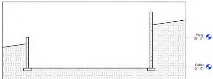
FIGURE 3.37 This section view illustrates how the building pad adjusts the extents of the topographic surface.
