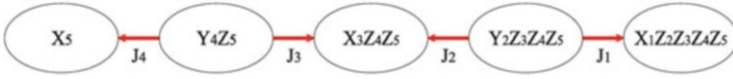
Fig. 4.2 Oriented graph representing the recurrence formulas needed to obtain the \hat{\mathcal{X}}_5(t) operator decomposition for a 5-qubit chain, whose Hamiltonian reads \hat{\mathcal{H}} = \sum_{i=1}^4 J_i (\hat{X}_i \hat{X}_{i+1} + \hat{Y}_i \hat{Y}_{i+1}) (Adapted from Int. J. Quant. Inf. 6 , Supp. 1, 659 (2008))
