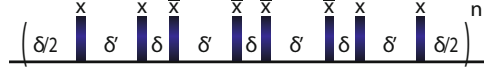
Fig. 6.7 NMR pulse sequence for the creation of the DQ Hamiltonian. Here we show a 8-pulse sequence used in the experiments to create the DQ Hamiltonian, generating the propagator U_{MQ}^x . Bars are \pi/2 -pulses along the x or \bar{x} = -x axis. The time delays between pulses are \delta and \delta' = 2\delta + w , where w is the duration of the \pi/2 pulses. Shifting the pulse phases by \pi/2 (that is, pulsing along y ) we obtain the propagator U_{MQ}^y = (U_{MQ}^x)^\dagger
